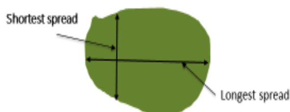
Figure 17. Diagrammatic representation of tree crown spread.
