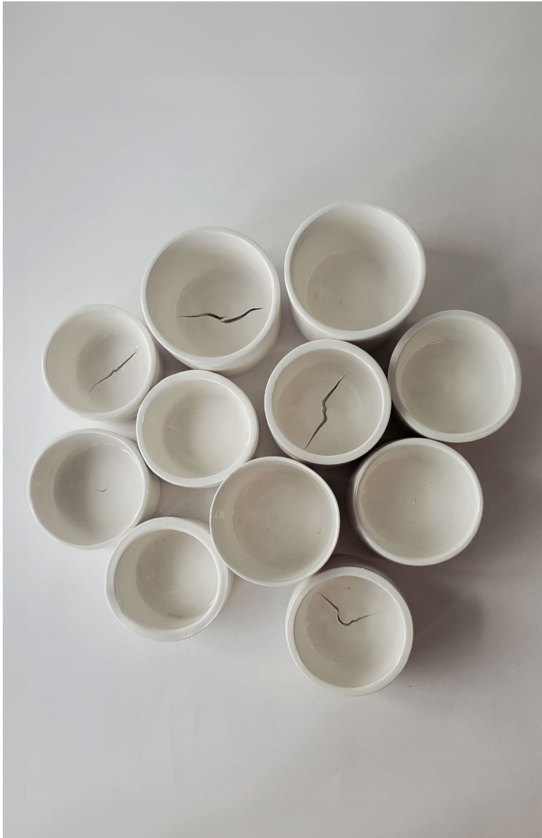
Figure 27. Joel White, high-fire porcelain clay cups in clear glaze with compression cracks, December 2023.
