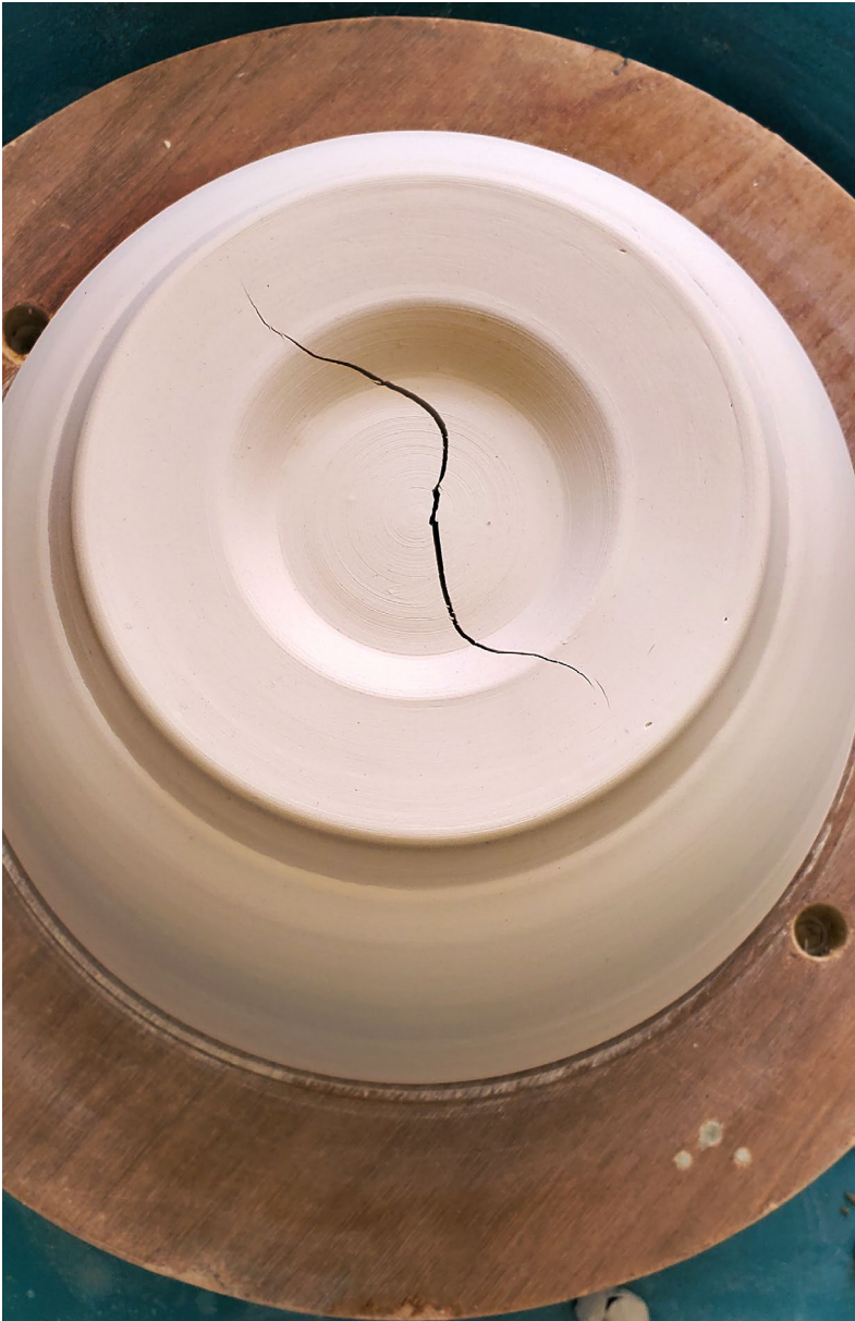
Figure 5. Joel White, mid-fire porcelain clay bowl with compression crack, dried on wheelhead, February 2024.
