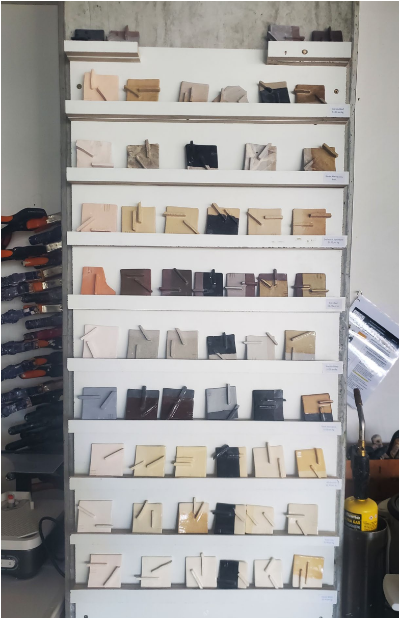
Figure 3. Joel White, Display of different clays with test glazes in the AUT Wet Labs, April 2024.
