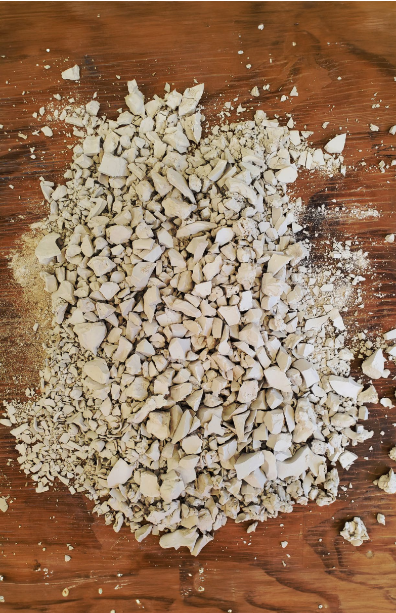
Figure 36. Joel White, Crushed porcelain pieces prior to being slaked with water for reclamation, January 2024.
