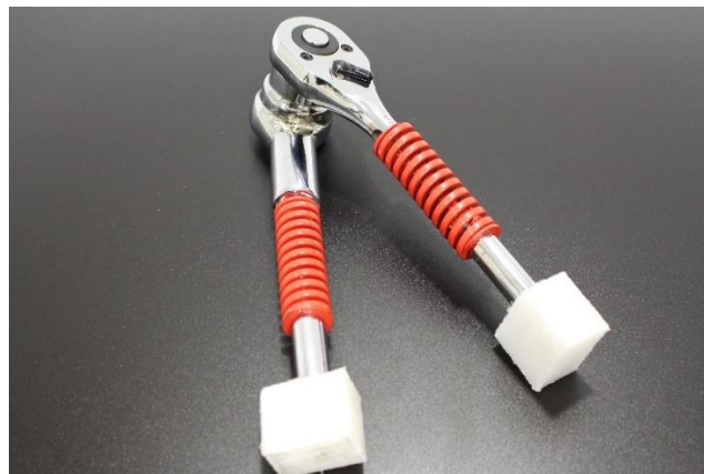
Figure 5.3-6 Assembly of Ratchet and Spring Joinery- without 3D printed housing
