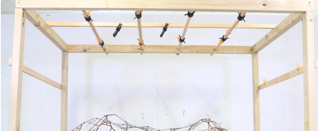
Figure 6.7-79 Marionette contraption - 3d printed parts assembled in frame
