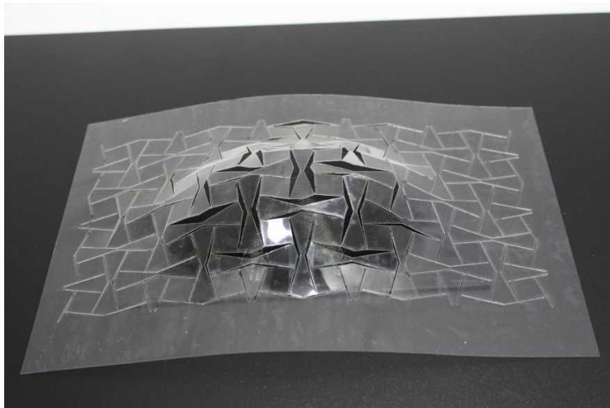
Figure 3.2-5 PETG- Lasercut trial of Rotating Square Auxetic on Ellipsoid Dome , laid on dome , dome removed
