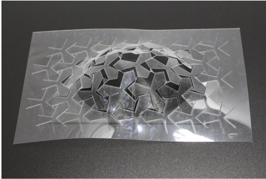
Figure 3.2-6 Lasercut trial of Rotating triangle Auxetic on Ellipsoid Dome , laid on dome , dome removed
