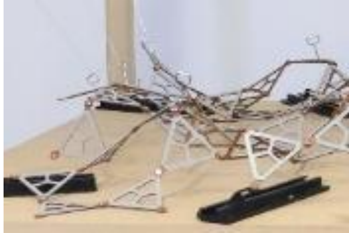
Figure 4.5-6 Unintended Vertical Piling of Units
