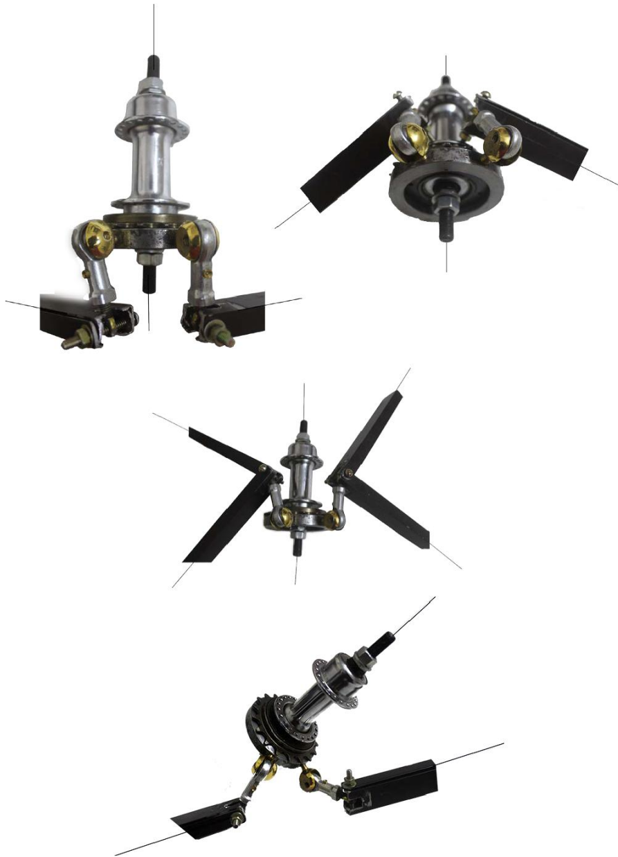
Figure 5.3-1 Physical Prototypes from Previous research- Junction Joinery Note: From , Deployable reciprocal shells through auxetic behaviour: Architectural hypothesis to fabricate double-curved structures by Jayachandran, S. (2019).
