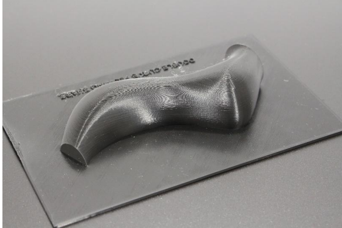
Figure 4.2-7 3d printed forms for testing - Double curve Flowing shape
