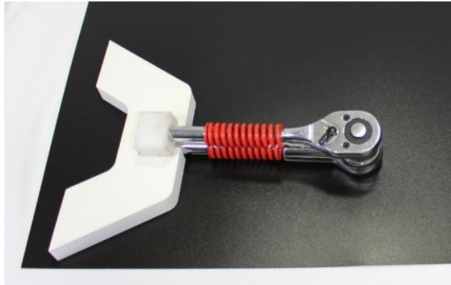
Figure 5.3-7 Assembly of Ratchet and Spring Joinery- with 3D printed housing
