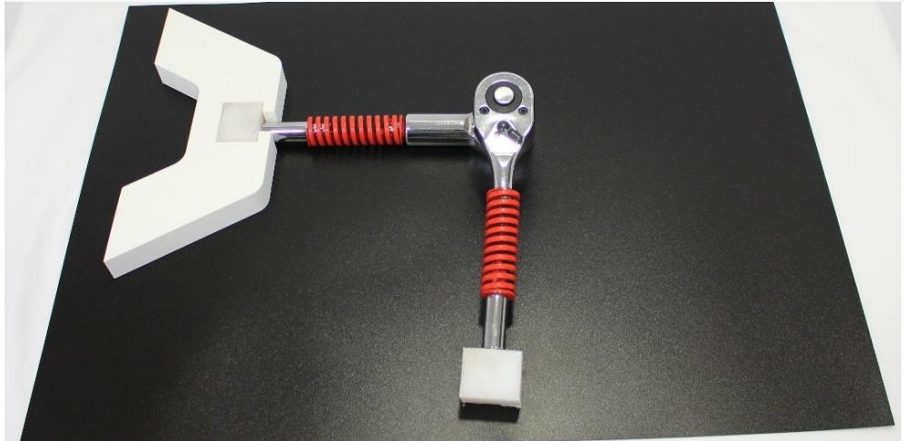
Figure 6.7-98 Testing of Ratchet and Spring Joinery in various degree of Yaw rotation
