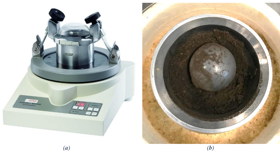
Figure 3.8: Soil sample preparation for elemental analysis; (a) FRITSCH Vibratory Micro-Mill "pulverisette 0" (FRITSCH, 2001), (b) pulverised soil sample.
