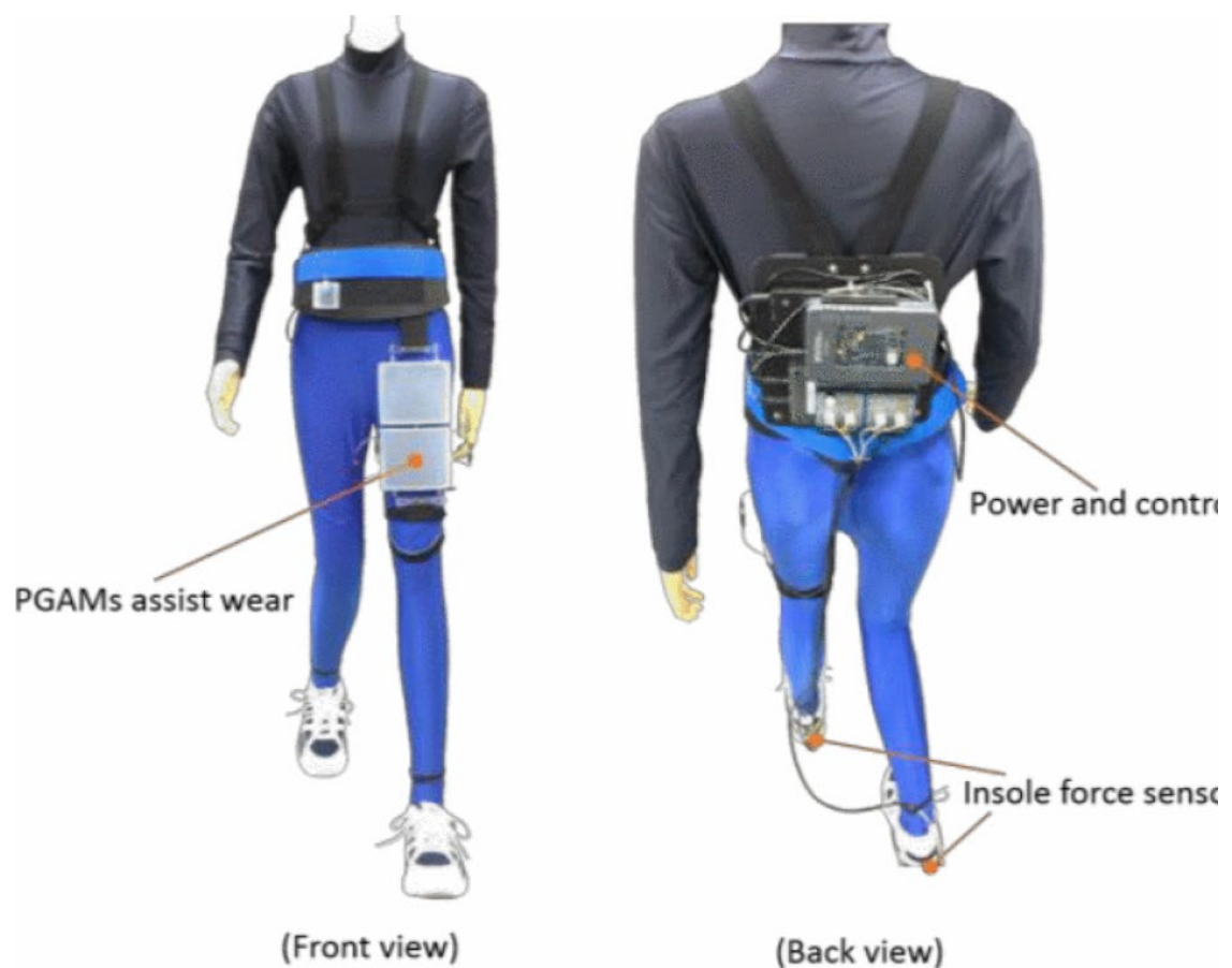
FIGURE 3.6 EXAMPLE OF AN SWRR BASED ON PVC GEL ACTUATOR. REPRODUCED WITH PERMISSION. [327] COPYRIGHT 2016, IEEE.
