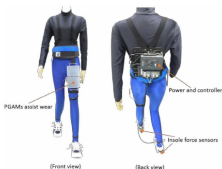
Figure 6. Example of an SWRR based on PVC gel actuator. Reproduced with permission. [138] Copyright 2016, IEEE.
