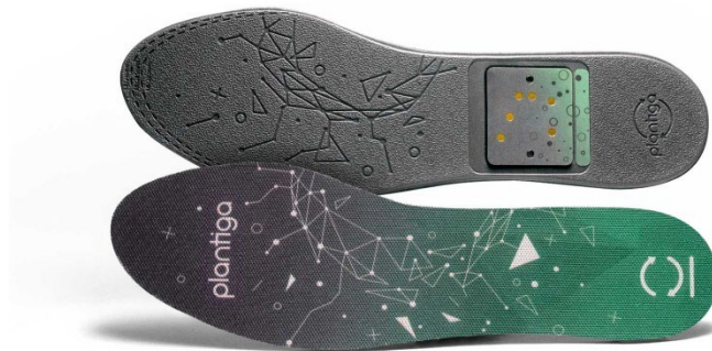
Figure 2: Plantiga inner sole and measurement unit.
