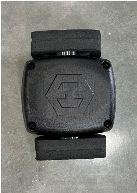
Figure 5. Strain gauge capable of measuring compressive force at 1,000 Hz.
