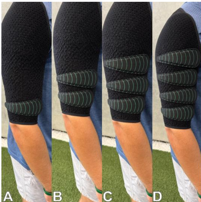
Figure 24. Above elbow loading using 100-g weights: 100-g (A), 200-g (B), 300-g (C) and 400-g (D).
