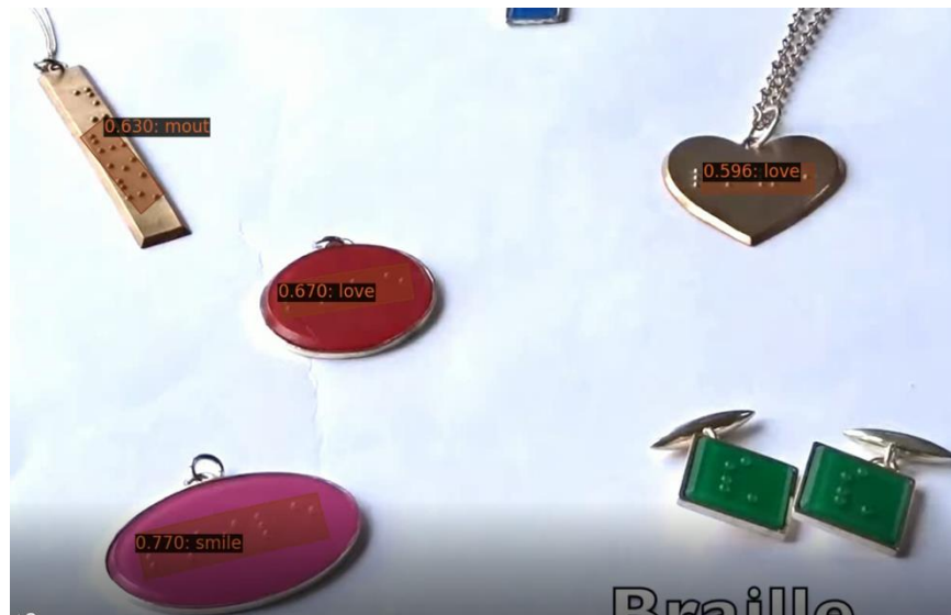
Figure 5.3: Mis-predicted and undetected braille
