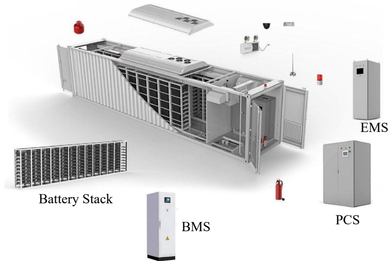
Figure 1.2 Schematic diagram of the key components of a BESS.
