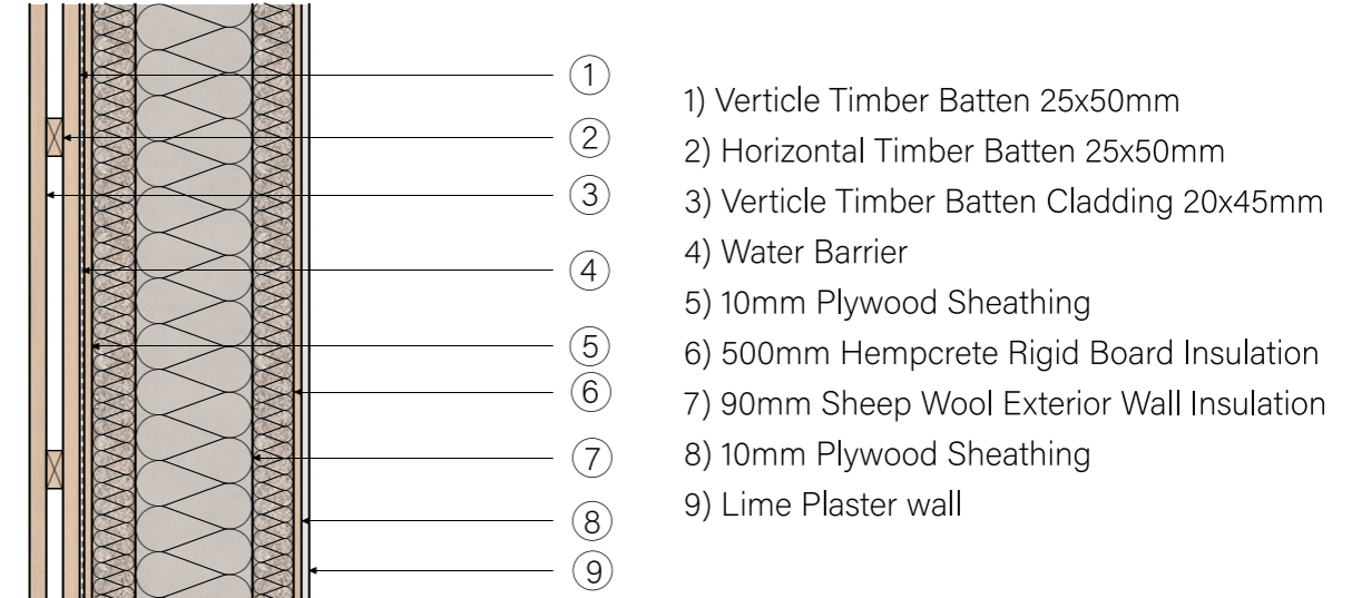
Figure 57. Timber Wall Detail Drawing Version One (Scale 1:200)
