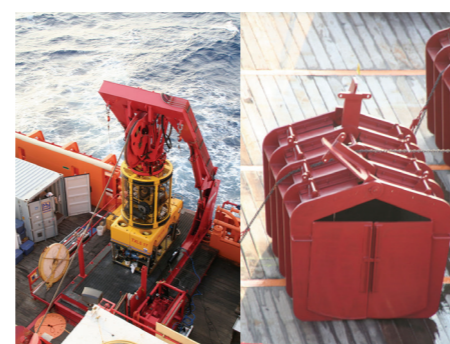
Figure 10 & 11: The Perry Triton XLS-17 ROV & Large Artifact Retrieval Tool (Irion, 2017, p332 & p335)
