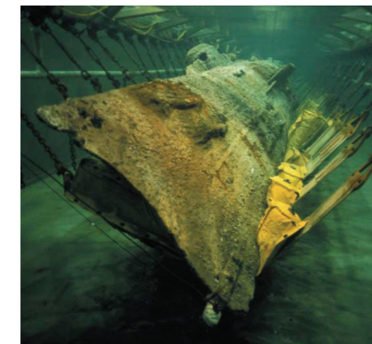
Figure 37: Hunley Resting in Its Tank with Anodes in The White Perforated Pipes at Warren Lasch Conservation Center (Michael, 2004, p140)
