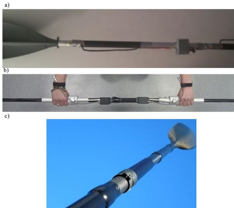
Figure 11. Previously studied instrumented paddle shaft designs
