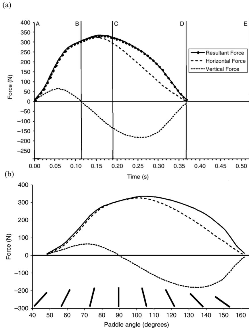
Figure 3. Blade force profiles of an elite kayaker
