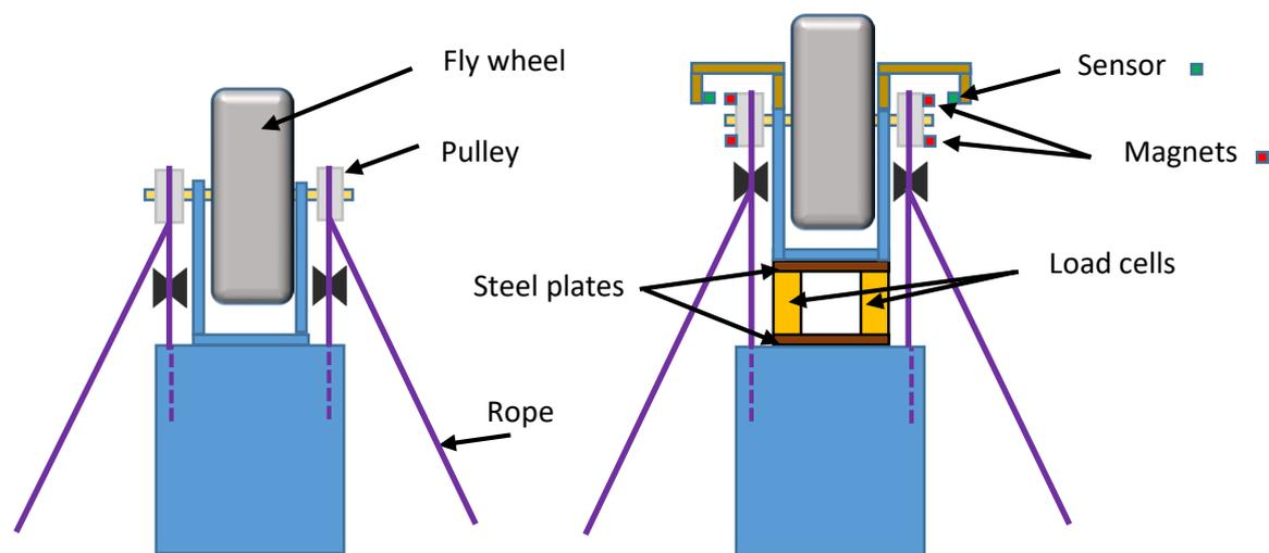
Figure 1. Kayak ergometer with load cells and wheel sensors
