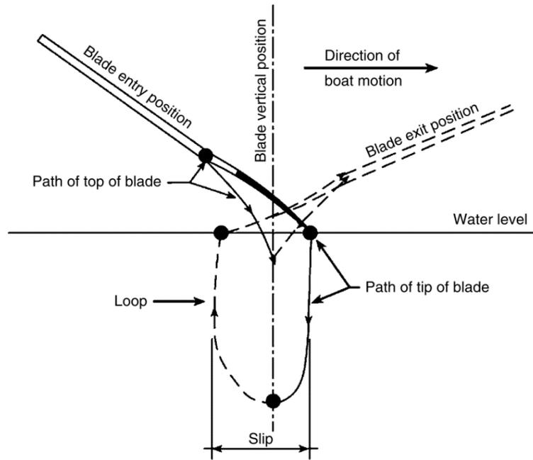
Figure 2. A sagittal view of blade-water dynamics during the paddle stroke
