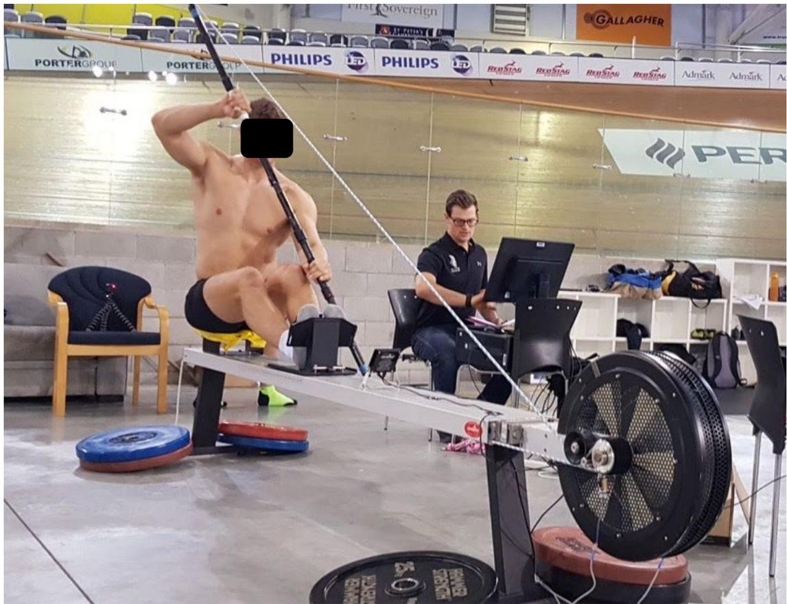
Figure 10. Kayak ergometer in use during CRNZ testing
