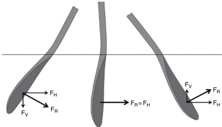
Figure 4. Blade force components at different paddle shaft angles
