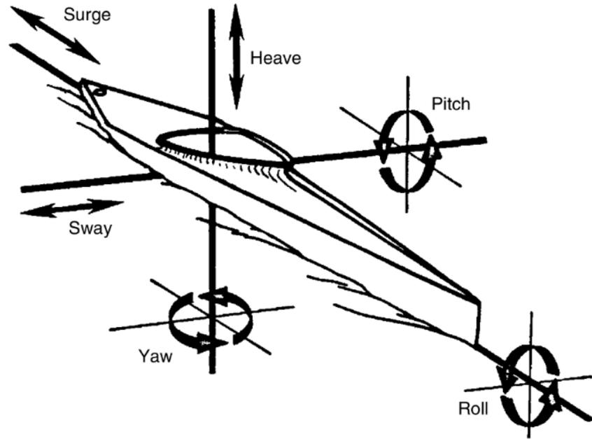
Figure 1. Boat movements of a kayak
