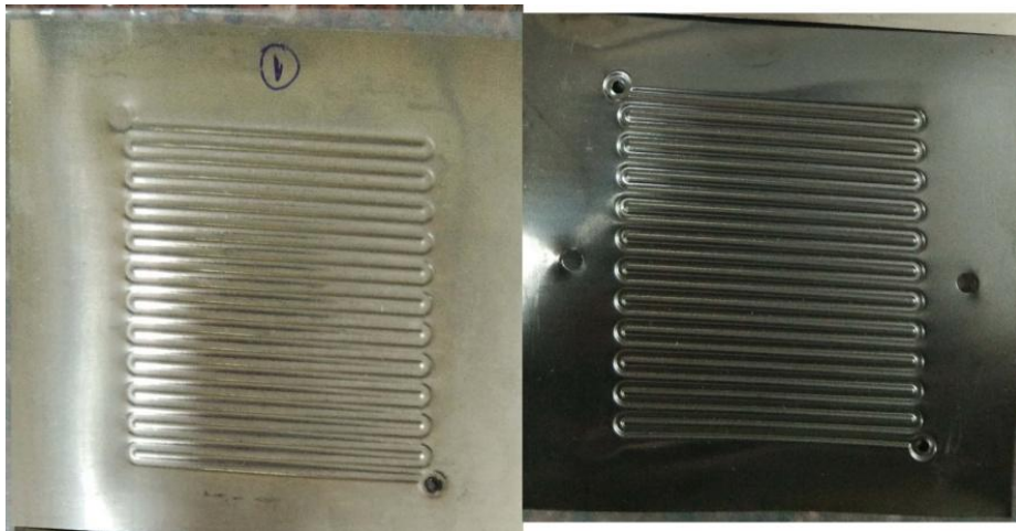
Figure 43: Photograph of Bare Titanium (Left) and WCC coated titanium plate(Right)
