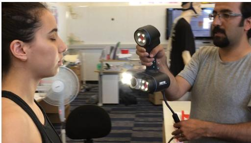
*Note.* Laser scanning of the lead actor's face (Melanie Mirfin) using GoScan (February 2018).
