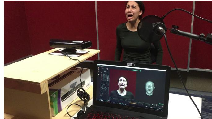
Dylen Velasquez (the production supervisor) capturing facial motions of Melanie Firmin (Stella's performance actor). This first phase of the facial capturing was realised using Kinect sensors before the facial data was sent into Maya for cleaning and adjustment. Later, TrueDepth sensors were acquired for the final facial capturing of the actors, as evidenced in the trailer.
