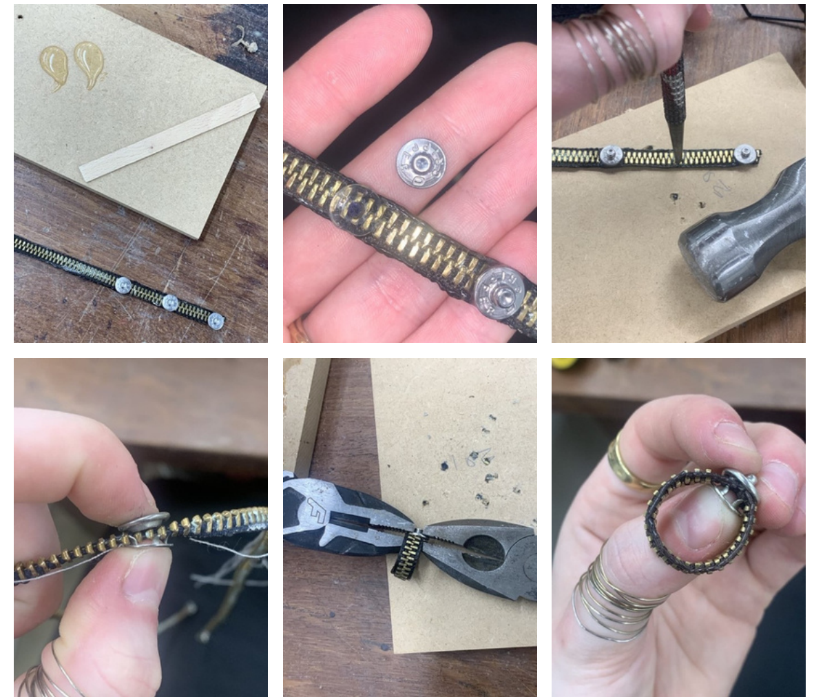
Figures 36. Glue Failure & Process Reconsideration, (Alix Vital, 2025).
