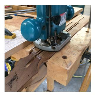
Figure 172. Using a router the truss rod and carbon fibre reinforcing slots are cut. The carbon fibre rod provides tremendous stiffness, lending strength to an otherwise light weight timber. Author's image 2017
