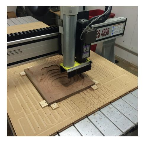
Figure 15. CNC Router machining back plate. Author's own image 2017
