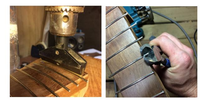
Figure 174. The fingerboard is laid out using the Laser cutter to engrave fret slot layout, which are subsequently cut by hand, the fingerboard is radius-ed, and the frets pressed in using an arbor in a drill press (left). The fret ends are trimmed (right) then leveled crowned and polished. Author's image 2017
