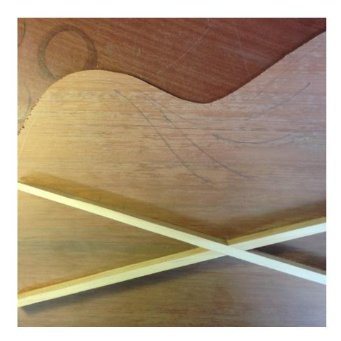
Figure 80. Totara soundboard with braces glued in place detailing the proposed positions for soundhole slots drawn on in pencil. This image was used to import into Rhino and create a drawing to map the slots and allow them to be cut in the Laser cutter. Author's image 2017
