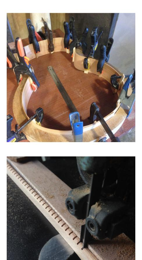
Figure 88. (Opposite top) The sides are soaked in hot water for 30 minutes then bent on a hot aluminium form the allow them to be clamped into a body mould where they will set over a 24 hour period. Author's image 2017
