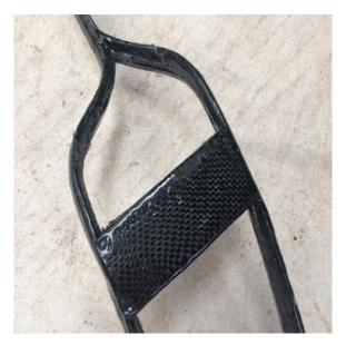
Figure 162(right). The part after curing, and before any cleanup, showing defects not only as a result of the vacuum bag, but also of the method of laying fibre on the frame. This would have caused issues with tolerance and fit against the CNC machined soundboard. Author's image 2017
