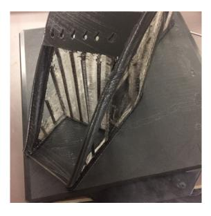
Figure 160. The first successful print had an error which the research deemed insignificant enough to proceed with. (The right hand leg has a deformation 10mm below the string harness) Author's image 2017
