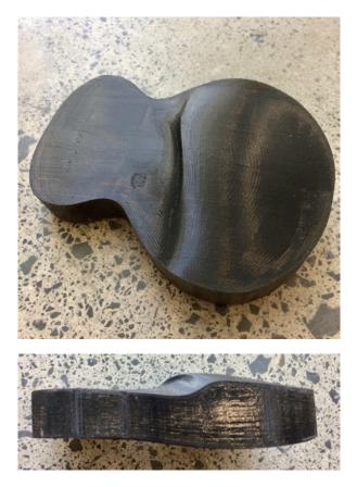
Figure 122 (above) and 123 (below) . 3D printed models with improved and softened contours. The model below shows a thinner body profile iteration. The same defect is visible at left in front of the wave contour, illustrating an error in the CAD drawing. Author's image 2017
