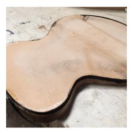
Figure 154. The carbon fibre strips are laid sequentially with little overlap around the rebate. The length allowed for a random start/finish with no weak points. Author's image 2017 Figure 155. The carbon fiber was laid up on its edge allowing it to tack onto the previous layer and the epoxy to flow down between, achieving a very high carbon to epoxy ratio, and greater strength. Author's image 2017
