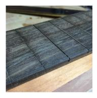
Figure 106. (right) Fret slots in the fingerboard, detailing laser engraved slots on the left and hand cut on the right. The CAD based layout helps determine critical spacing which influences whether the instrument will play in tune. Author's image 2017
