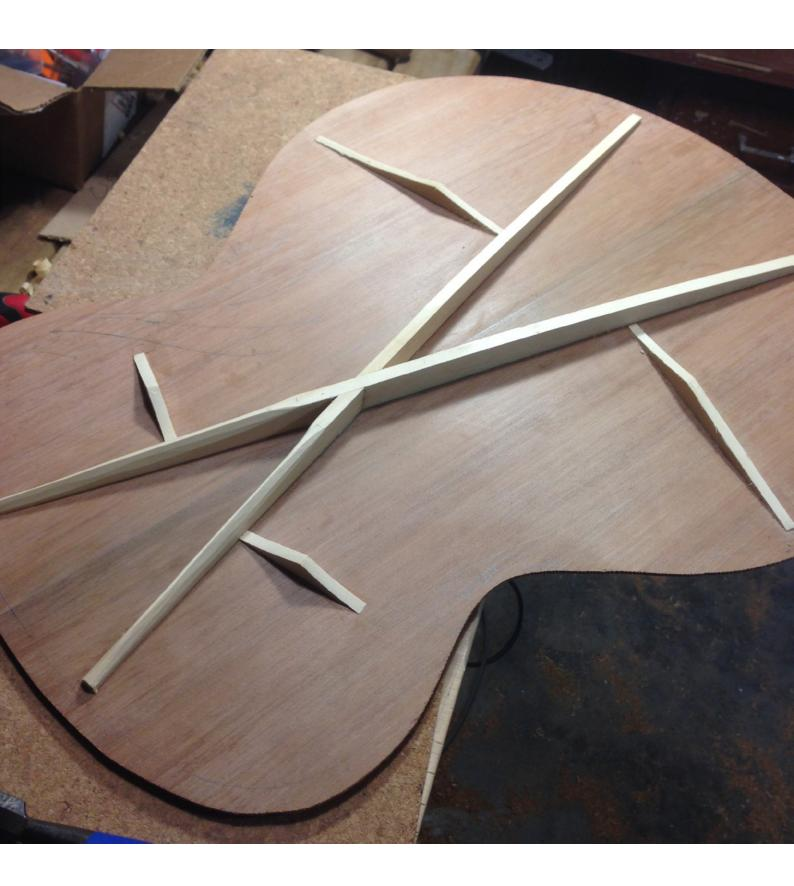
*Figure 83. (Opposite top) Back plate having been joined, trimmed and the back grafts have been glued in leaving space for the back braces. Author's image 2017*
