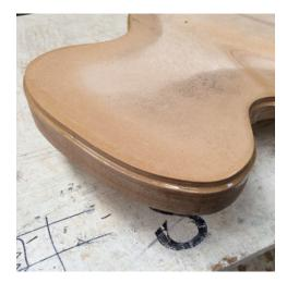
Figure 152. The rebated perimeter of the center section of the mould is coated with epoxy resin and left to set up for around 2 hours to become tacky. Author's image 2017
