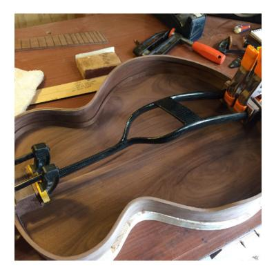
Figure 169. The bracing was laid up and trimmed to fit between the neck and tail blocks, and walnut face plates were cut to house the ends of the bracing legs. This assembly was glued in place with epoxy resin. Author's image 2017
