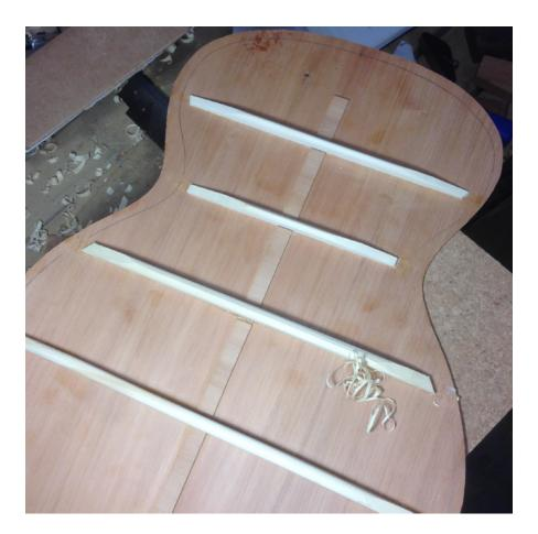
*Figure 86. (Opposite top) Planing the back braces to remove excess material, which allows them to be lighter weight but just as stiff. Author's image 2017*
