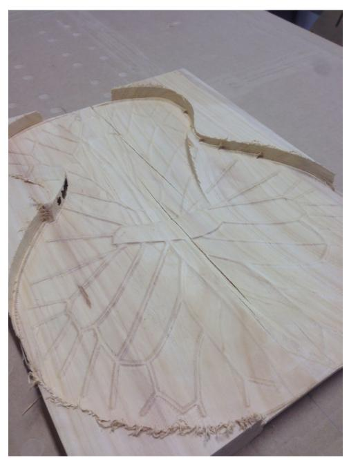
Figure 28. Finished veined soundboard with cracks - commercially unusable, the natural faults in the timber have been exposed due to the design and machining used. Author's image 2017
