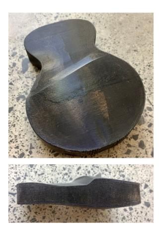
Figure 121. 3D printed model with angular contours. The model was re drawn to remove the hard contours Author's image 2017
