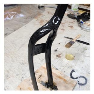
Figure 164 (right). The frame on a support rig, allowing epoxy to be applied and then tack up creating a far better carbon fibre layup. In this image there has already been one layer applied, a total of 4 layers were built up. Author's image 2017
