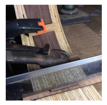
Figure 137 (above) After the sides are bent into shape the ends are trimmed and glued together inside the body mould, which was machined on the CNC. Author's image 2017
