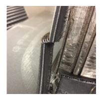
Figure 159 (above). Initial printing on the Makerbot Z18 failed due to poor support structures, but with some fine tuning began to yield satisfactory framework for carbon fibre. Author's image 2017
