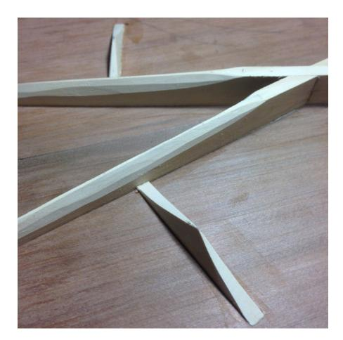
Figure 81. Detail of the bracing members on the Totara soundboard. The same level of complex carving, tapping and listening was involved in creating an optimal soundboard, one which would resonate as freely as possible without deforming under string pressure. After the carving procedure, the braces are sanded to achieve a uniform taper and parabolic profile Author's image 2017.
