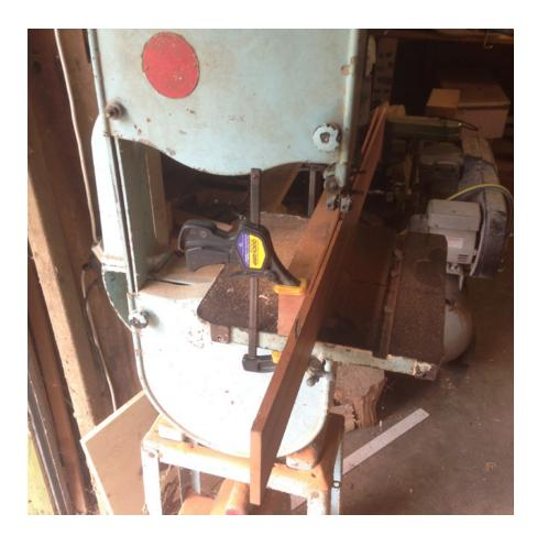
Figure 78. Matai being band sawed for the sides of the flat top guitar. Author's image 2017
