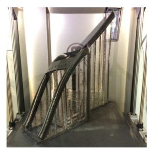
Figure 163(left). A successful print on the buildplate of the Z18, this frame printed better due to modified supports around the lowest parts of the build. Author's image 2017
