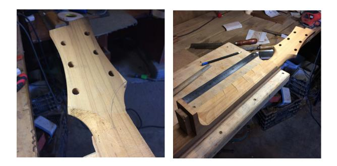
Figure 175. A process which in industry would be automated, but at this prototype stage is still hand made; shaping the neck. Pencil drawn lines, rasps and files are used to define the neck contours and taper. Author's image 2017
