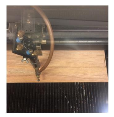
Figure 135 (above) Laser cutting the profiles for the sides in Rata. The profile was extracted from the CAD model, having a flowing contour unlike traditional guitars. Sides were also cut in walnut, which was used in the final model after defects were found in the Rata. Author's image 2017
