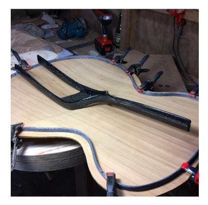
Figure 167. Above, the bracing resting in approximate place with the edge beam temporarily clamped in place. Author's image 2017
