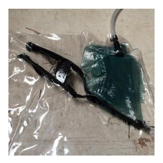
Figure 161 (left). Vacuum Bag infusion of carbon fibre onto 3D printed frame. The pressure of the vacuum bag not only removes air, and sucks the fibre down onto the model, in this case it also distorted the right leg, at the point where the defect had been previously noted. Author's image 2017
