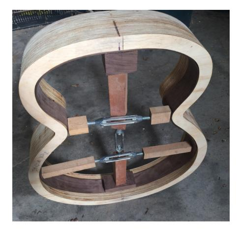
Figure 139 The sides, neck and tail block assembly held in place inside the body mould. This part of fabrication is very labour intensive, taking place over three days, with a full day for drying after steam bending. Author's image 2017
