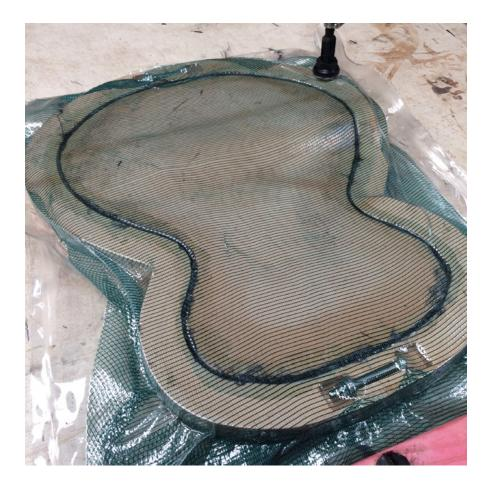
Figure 150. Revised edge beam three part mould. The outer parts of the mould are separated by loosening the bolts, allowing them to be easily released from the center section. Author's image 2017
