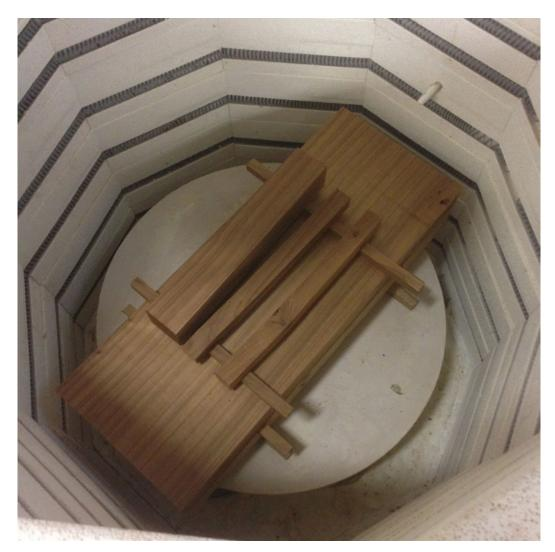
*Figure 51. The first torrefaction tests took place in a ceramics* kiln, but issues arose with smoke and the treatments were discontinued. Relocated to the researchers site, further tests were conducted in a domestic oven, which functioned in a way so as to minimise direct heat at the ends of the timber stock, an area vulnerable to smoldering. Author's own image 2017
