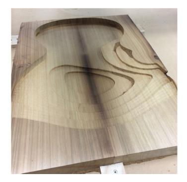
Figure 128 (above) Cypress blank after internal horizontal roughing pass, ready for finishing pass and string hole detailing. Author's image 2017
