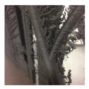
Figure 39 (above), Figure 40 (left). 3D printing on the Makerbot Z18 with CFPLA. Support structures and filament ooze at left and complete failure above due to an extrusion error later traced to how code was written by the software. Failures with this scale of printing lead to questions around the abilities of the printer and software, with uprades being made to both. The CFPLA was more rigid than the standard PLA but showed susceptibility toward fracturing. Author's image 2017.
