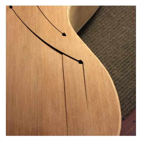
Figure 109. Flat top guitar with cracks emanating from the sound slots following the grain - a very disappointing and disheartening occurrence. Author's image 2017
