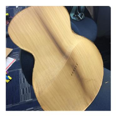
The process for machining the back plate was the same as the soundboard, and multiple backs were made from Native Rata and American Walnut. The choice to make multiples was initially based on the idea of making two near identical models with variations in soundhole positioning and design, but issues with machining the Rata lead to using Walnut as an alternative.
