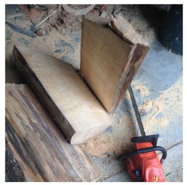
Figure 49. Cypress harvested and seasoned by the researcher, Each section was split and quartered to yield the most consistent grain orientation. Author's own image 2017
