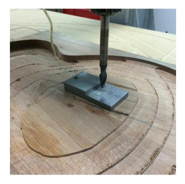
Figure 133(above) Tool being zeroed on the top of the blank, by being lowered onto a touchoff plate, allowing for the most accurate cut possible. Author's image 2017
