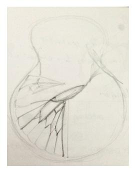
Figure 21 (above). Initial concept sketch of insect veined soundboard - the idea of a strong skeletal frame supporting a membrane like 'skin' of timber. Author's image 2017.
