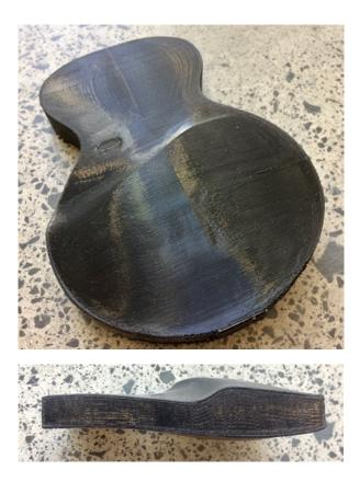
Machining the soundboard began with the cypress blanks after thermal modification (fig 124), they were planed to thickness, glued together and positioned on the CNC.
