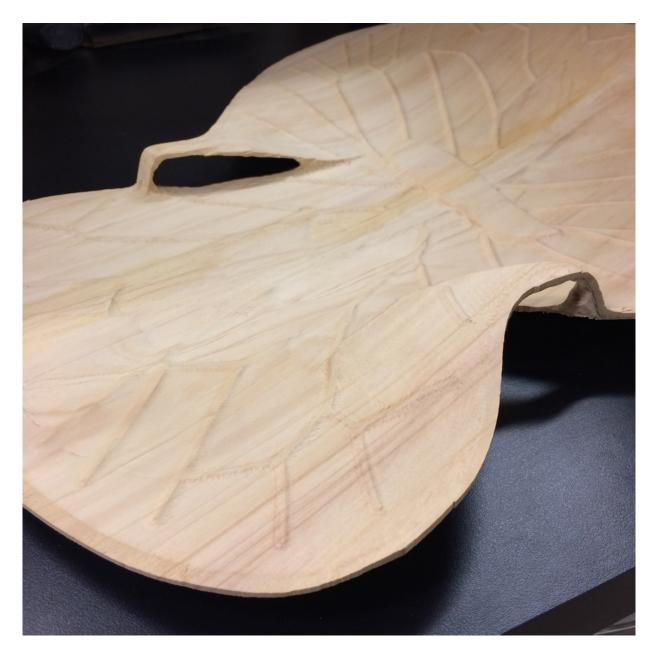
Figure 30. Veined soundboard with soundholes cut, and cracks glued to allow for tap tuning and 'loosening'. Author's image 2017
