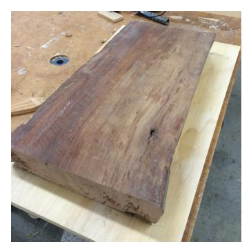
Figure 130 (above) River salvage Southern Rata hot glued onto a plywood sled for machining. This process levels the blank and allows for parallel faces, and accurate CNC machining. Author's image 2017
