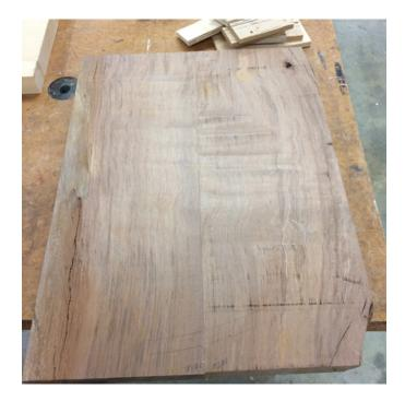
*Figure 131 (above) Rata blank glued together to match figure (horizontal bands) Author's image 2017*
