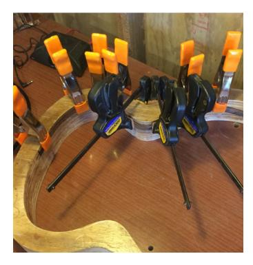
Figure 140. Steam bending the linings and clamping them into the body mould. Author's image 2017
