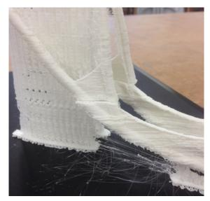
Figure 37 (above), Figure 38 (right). 3D printing on the Makerbot Z18. The model was printed on an angle so that it would fit within the build volume. Issues with poor printing resulted from the size of the model and its inclination to flex and move under the extruder. Author's image 2017
