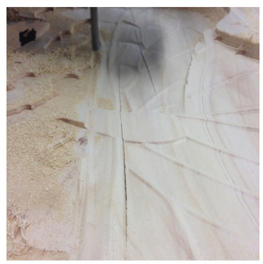
Figure 27. Parallel finishing pass - veined soundboard. Note cracks down the center. Author's image 2017
