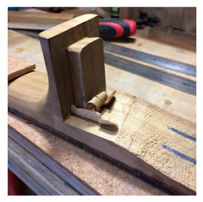
Figure 176. The neck dovetail tenon and extension are hand carved to fit the soundboard. Author's image 2017
