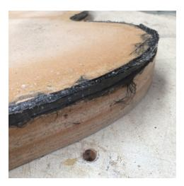
Figure 156. After curing overnight the outer mould was removed revealing the consistent impregnation of epoxy resin. Author's image 2017
