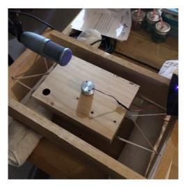
Figure 48. Isolation test rig. Boxes were suspended with rubber bands to isolate from external sympathetic vibrations. At the center of the test box is the bone conductor transducer, used to transfer sound to the soundboard. (2017 Author's image)
