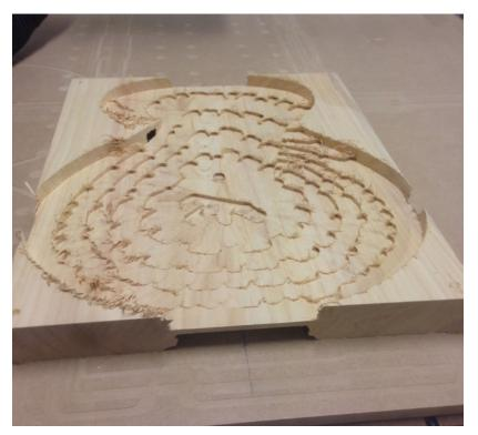
Figure 26. Finished roughing pass, not complex stepping pattern to allow for veining. Author's image 2017
