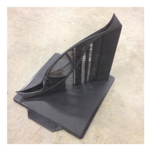
Figure 41. Successful print in CFPLA, due to modifications in the software and setup. This model does not have the structural stability to be included as part of the instrument Author's image 2017.
