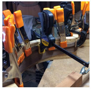
Figure 142. Gluing in the linings. This critical process holds the outside profile for the sides of the guitar, especially adjacent to the soundboard which does not make contact. Author's image 2017
