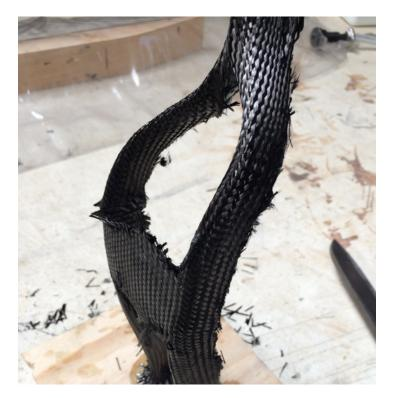
Figure 165. Above, the frame with carbon fibre cloth laid over tacky epoxy, before fresh epoxy resin is brushed on and worked in. Author's image 2017
