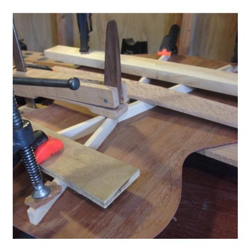
Figure 79. 'X' Braces being glued in place. Kahikatea was used for the braces, an analogue for spruce which would traditionally be used. The bracing pattern was chosen knowing the strings would not be fastened on the soundboard like a traditional flat top, instead they would pass over the bridge exerting pressure rather than shear force. This allowed for a lighter bracing option, one which would make room for the soundhole slots. Author's image 2017
