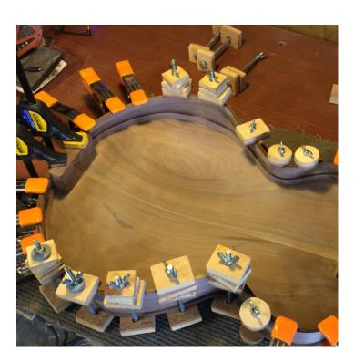
Figure 143. The back plate being glued to the side assembly. Author's image 2017
