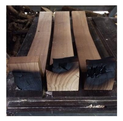
Figure 52. Neck blank torrefaction experiment failure. The end grain cracks proved to be vulnerable to smoking, rendering the neck blanks unusable. Author's image 2017
