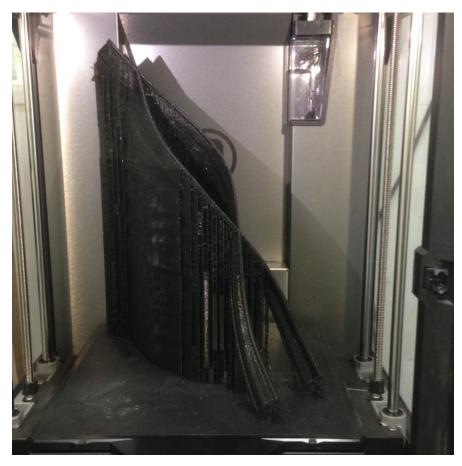
Figure 19. 3D Printer (Makerbot Z18) having completed a bracing model. Author's own image 2017
