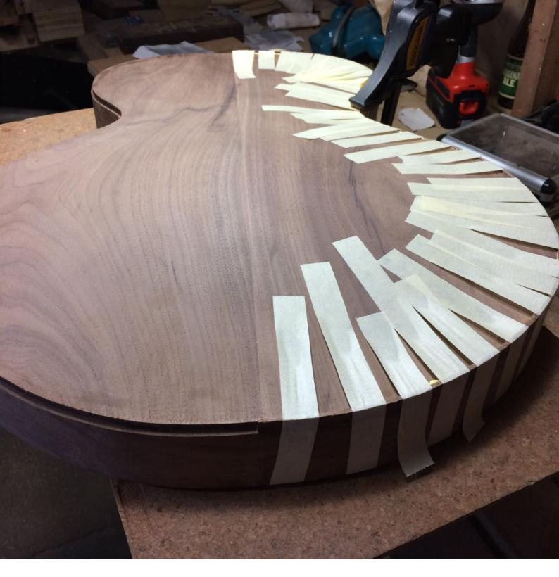
Figure 145 (above). Walnut binding being glued in place using masking tape to help conform to the contours. This was a very testing process - in many places the contours made fitting the binding very difficult. Author's image 2017
