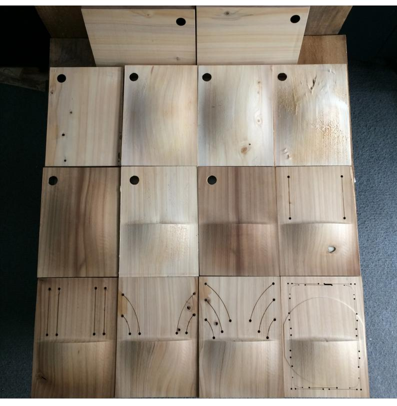
Figure 180. The box test soundboards (the floating soundboard was conceived after this photo was taken). Author's image 2017
