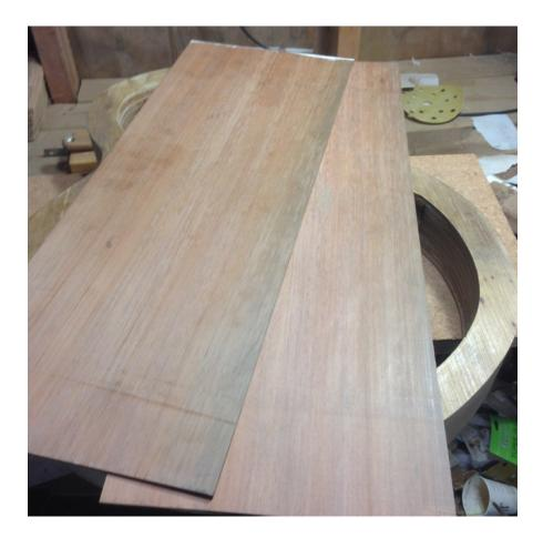
Figure 76. River salvage Totara soundboard timber. Discoloration on the right of the boards is caused by years of submersion in river water and silt. Author's image 2017
