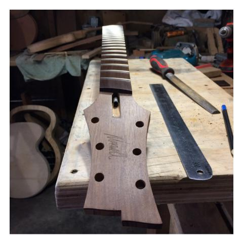
Figure 171. The neck was cut to profile from thermally modified cypress, using a template laser cut from the CAD model. The headstock facing and fingerboard were laser cut from thermally modified Rata, allowing for precise machining and placement. Author's image 2017
