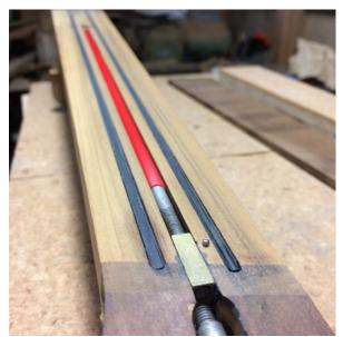
Figure 173. The truss rod (center in red) allows adjustment of the neck by resisting string tension. It is arguable whether it is necessary with the carbon fibre reinforcement. Author's image 2017
