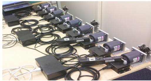
Figure 2. Multiple motor fault signature testbed.
