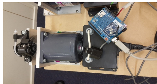
Figure 3. Arduino setup for wireless current monitoring.
