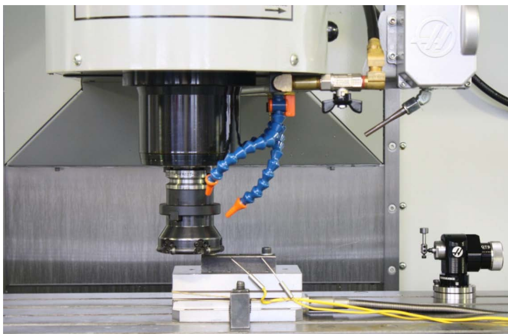
Figure 42: Experimental set-up milling trials - grade 1200
