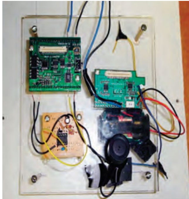
Figure 2.41 Components of a CO-WSN unit [66].
