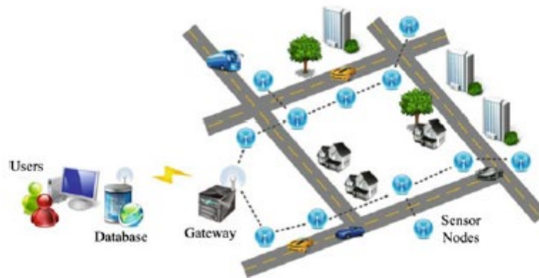
Fig. 8 Micro-scaled air quality monitoring system architecture [18]
