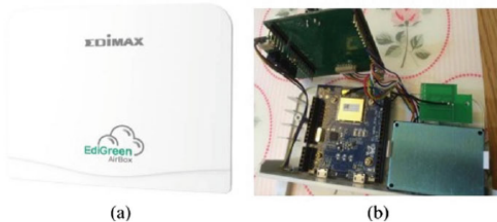
Fig. 11 AirBox device: a overview and b internal components [27]
