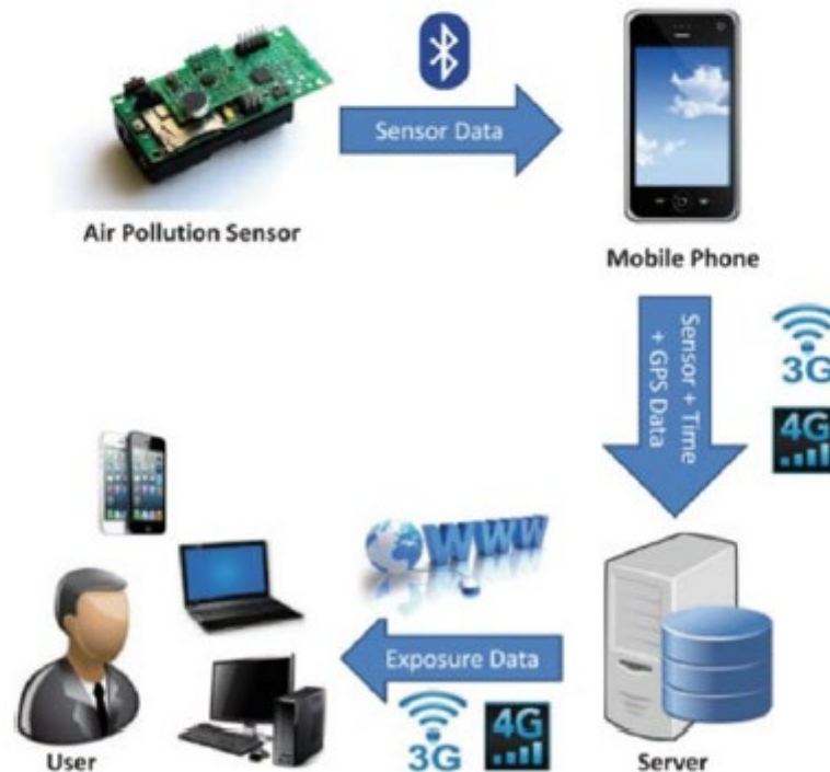
Fig. 9 HazeWatch system architecture [19]
