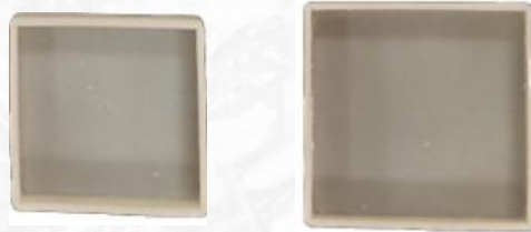
Figure 24. 8 cm x 8 cm x 2 cm and 10 cm x 10 cm x 2 cm size casting
