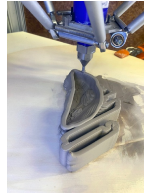
Whakaahua 46. Pito 1, without internal supports, with Matt-made 42 external support.
