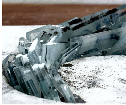
Figure 44. M Refiti. Packed fuzed glass before firing. E19 - Cast Glass Series, 2024, Photography.
