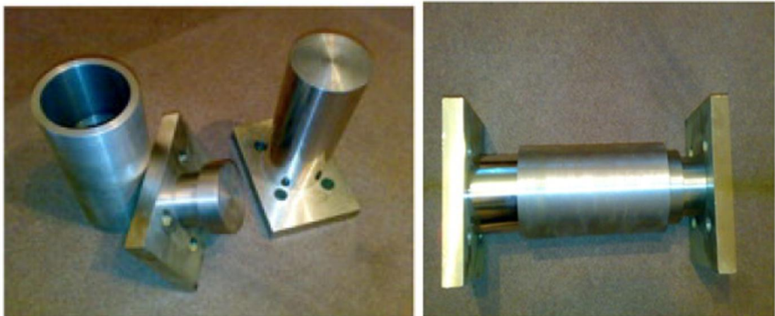
Figure 2-20 Cylindrical friction damper concept (adapted from Jaisee et al., 2021)
