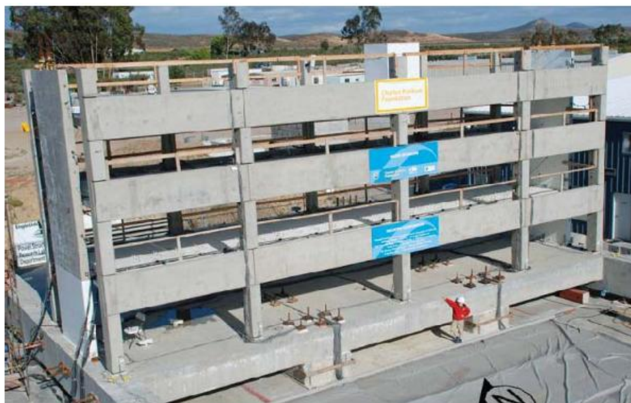
Figure 5-33: Shake-table test of DDSM precast building at San Diego (Schoettler et al. 2009)
