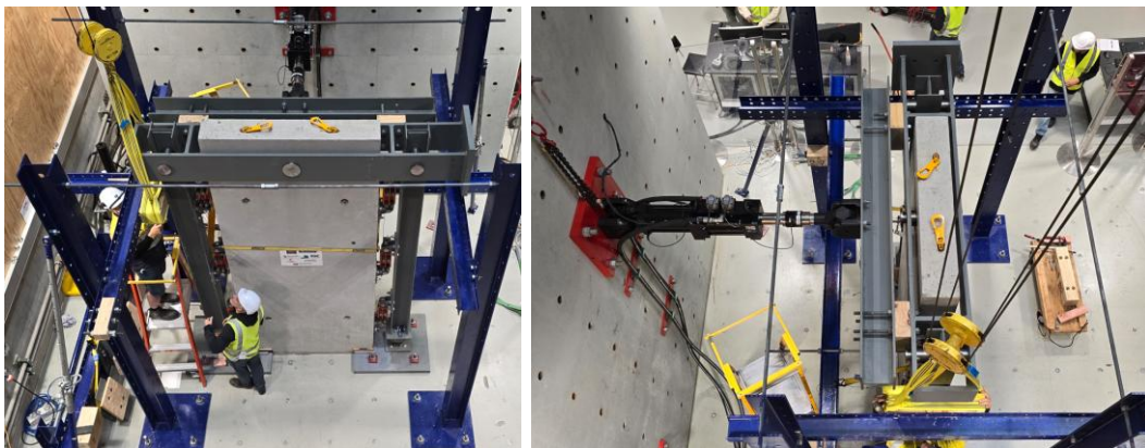
Figure 5-23: Concrete wall Out of plane loading setup
