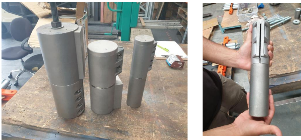
Figure 6-10: Scaled variations of RSFD tailored to tank conditions and capacity design specifications
