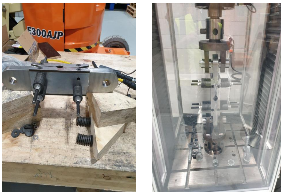
Figure 5-8: Assembling and testing of RSFJ units.
