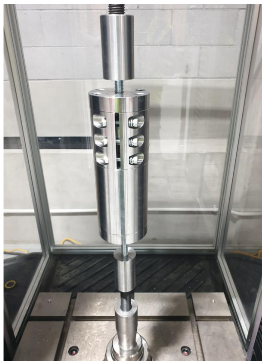
Figure 6-4: Assembled RSFD Prototype Undergoing Testing in Universal Testing Machine (UTM)
