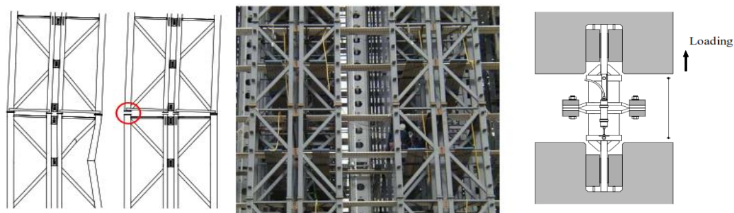
Figure 2-7: (a) Frame with conventional columns; (b) Frame with stepping columns; (c) industrial building Japan; (d) connection splice (Wada, Yamada et al. 2001)
