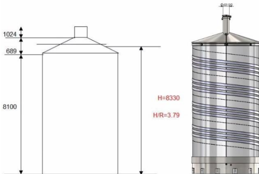
Figure 6-17: Schematic view of 125 KL wine tank
