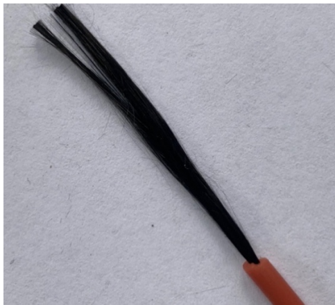
a) Silicon rubber covered carbon fibre
