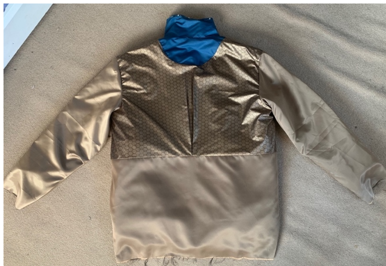
d) Process of connecting the lining shell with an outer shell (back)
