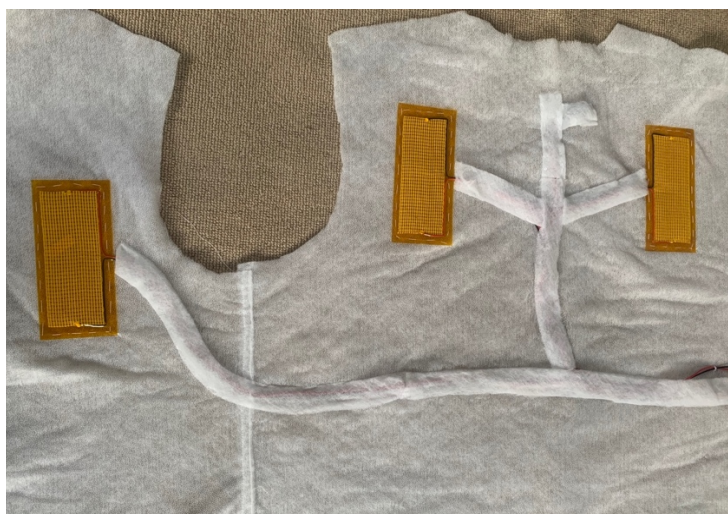
d) Covering wires with a strip of insulation
