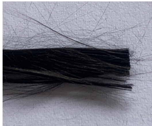
b) Carbon fibre (silicon rubber was removed)
