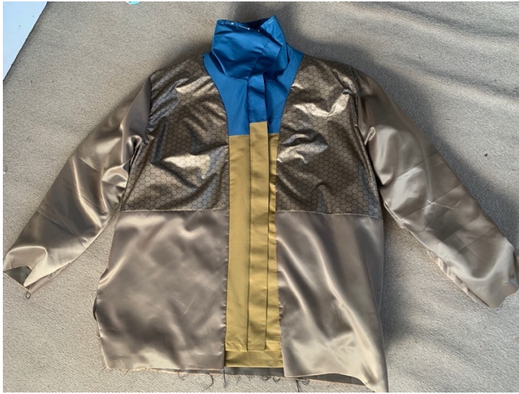
a) Process of connecting the lining shell with an outer shell (front)
