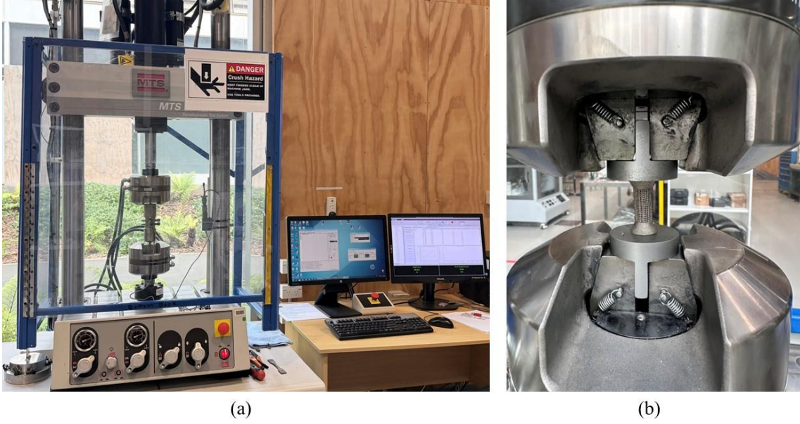
Fig. 3.5 Set-up of the fatigue tests: (a) Landmark Servo-hydraulic Test System and (b) [001]//LD lattice under compressive cyclic loading
