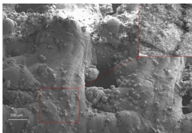
Fig. 7. Scanning Electron Microscopy image of polypyrrole coating on the printed stain-less steel 316L electrode at 150 X and 20 kX (inset) magnifications.
