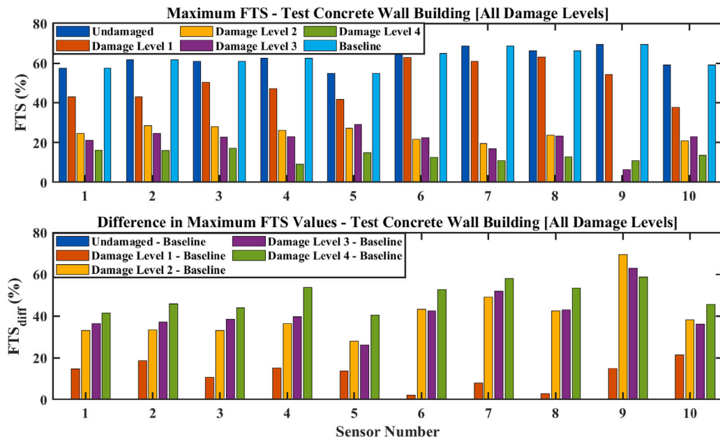
Fig. 18. Maximum FTS values and the difference between these values and the baseline, FTS_{diff} , for different damage levels at the location of each sensor for the 10 selected sensors on the test two-story concrete wall building under Medium-Level PGA .
