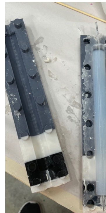
Figure 36. Open mould after the silicone set. Demonstrating how the mould worked with the wire being held at the bottom.
