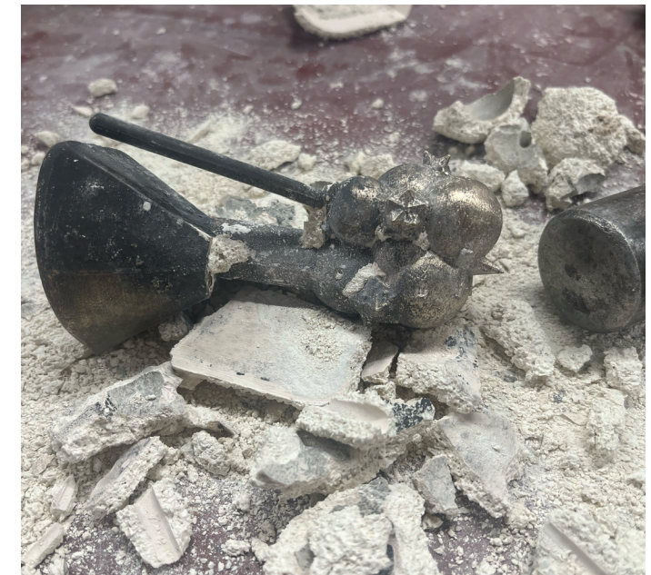
Figure 73. Removing ceramic shelling off the bronze object.
