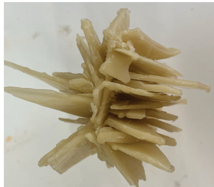
Figure 84. Wax shard ball before getting a plaster silica mould around it
