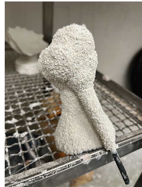
Figure 72. Ceramic shelling process over 3-D printed object.
