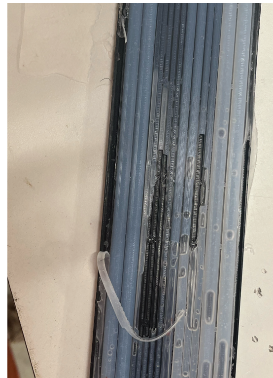
Figure 78 Silicone strings getting air bubbles from syringing in the silicone into the mould.
