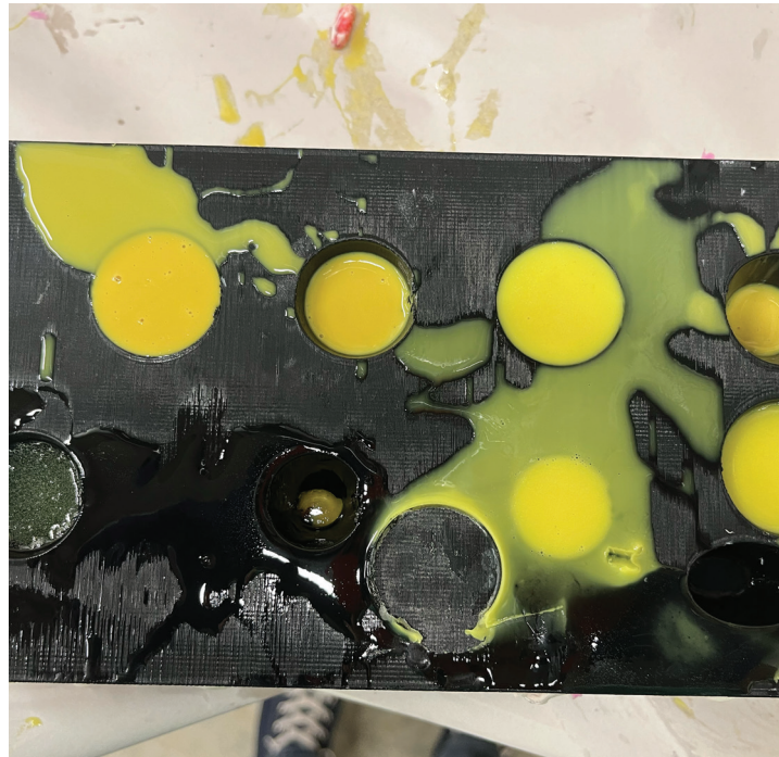
Figure 89. Different flexicast grades leaking into each other as mould did not close properly.
