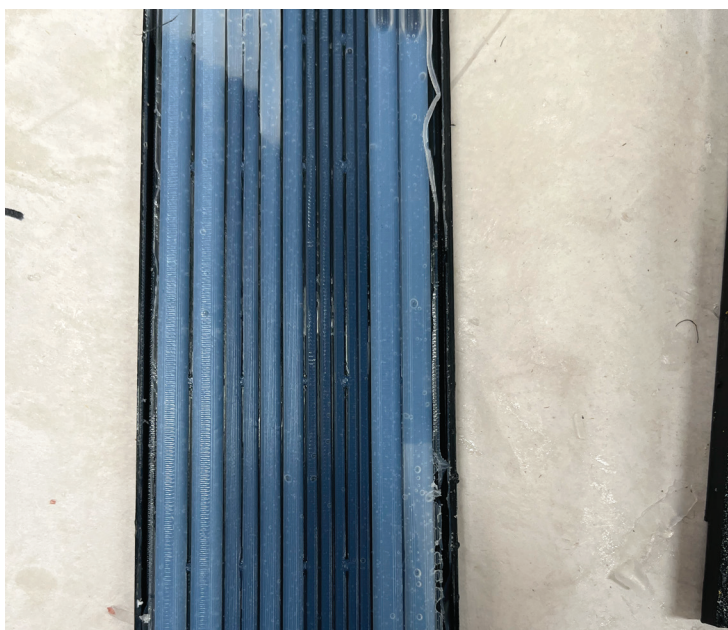
Figure 77. Silicone sinking to the bottom after pouring, then putting together, the two part mould.
