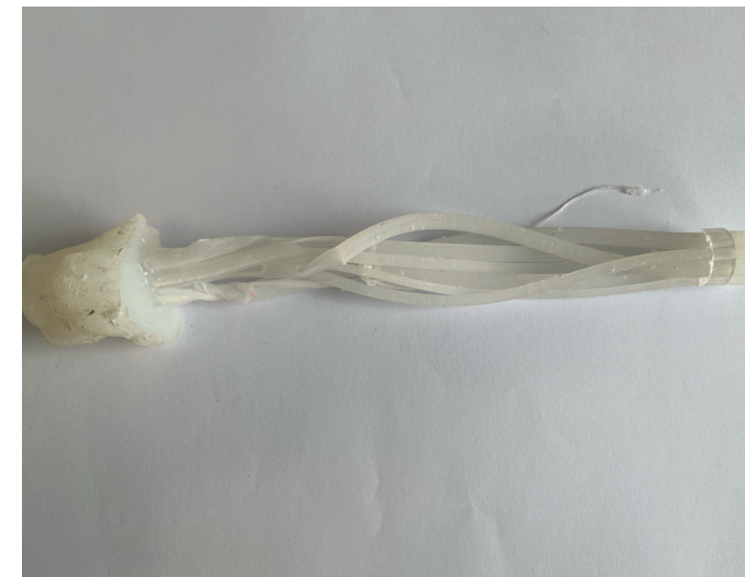
Figure 79. RTV handle with laser acrylic plastic holder on the other end
