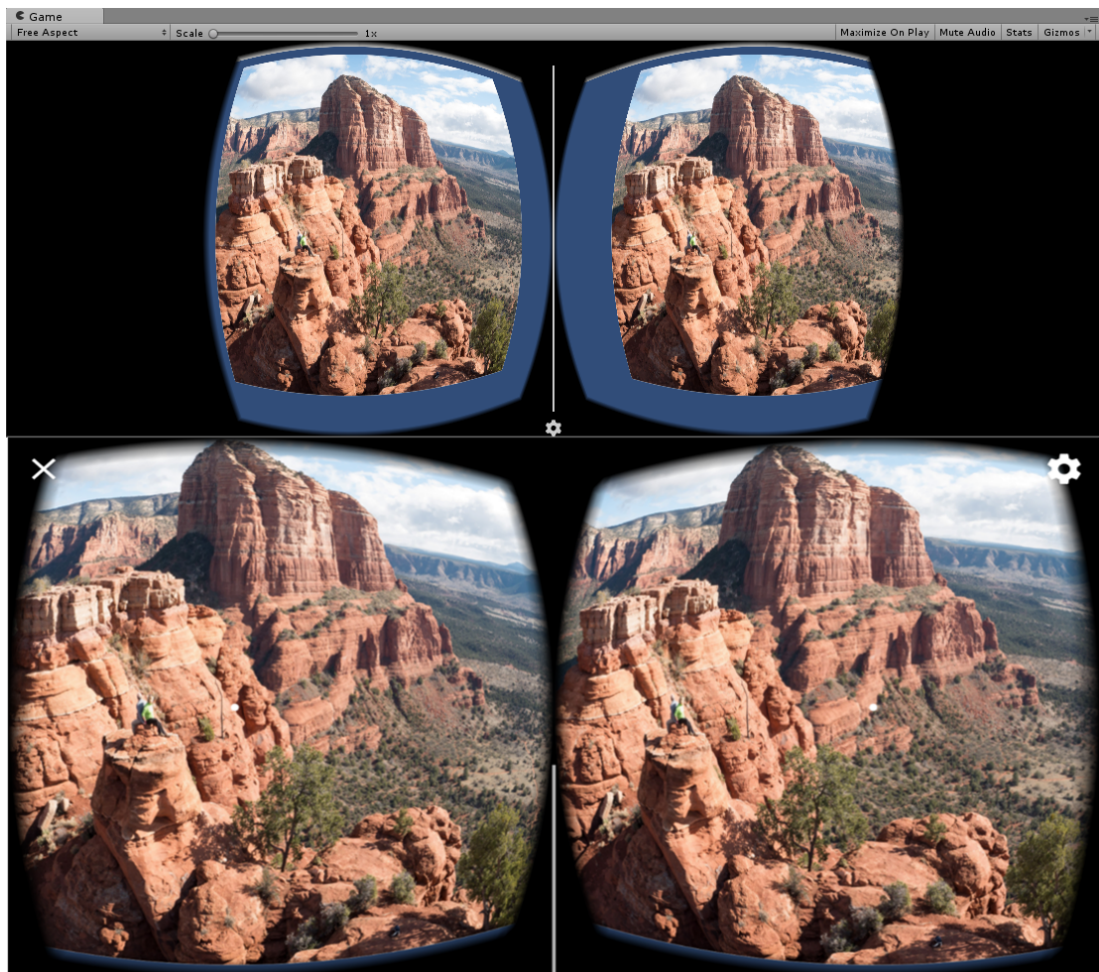
Figure 6.12: The camera display area in Unity preview mode(top) has different characteristics from the one in Android environment (below).
