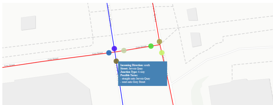
Figure 7. Interactive junction visualisation showing turn possibilities at a 4-way intersection. The tooltip displays available turns for Jervois Quay. (Colour Legend: Blue lines = North/East-bound traffic; Red lines = South/West-bound traffic; Distinct coloured nodes = Turn possibilities).
