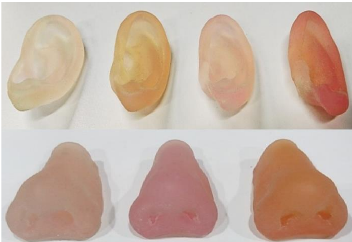
Figure 2.3. Printed prostheses with different material combinations (Tango Plus, VeroMagenta and VeroYellow)(Mohammed et al., 2016).
