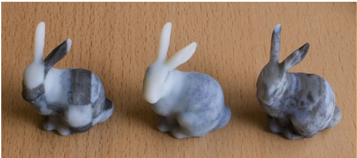
Figure 2.4. 3D printed example with specified subsurface scattering (Hašan et al., 2010).
