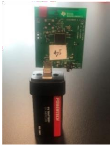
Fig. 5. TI CC2538 board with Micro USB
