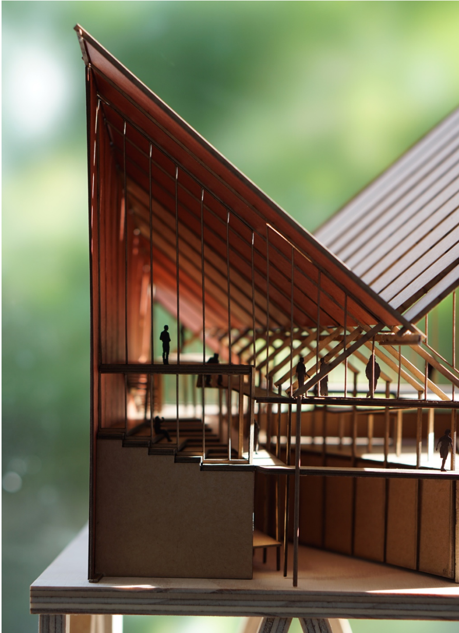
Figure 37. Kang, Taewoo. Proposed Design . 2017. Cardboard laser cut assembly.
