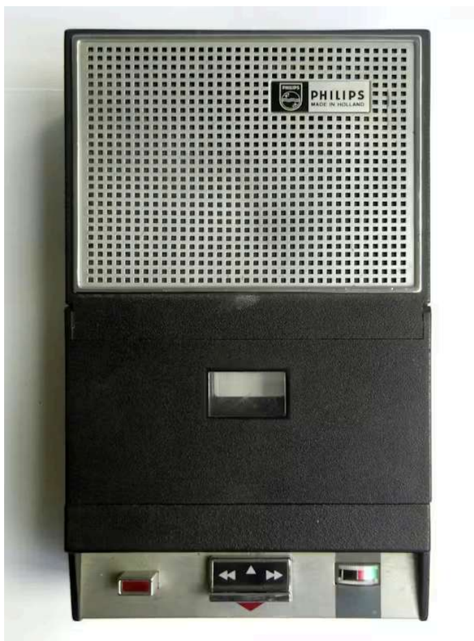
The Philips EL3300 was the first mass-market compact cassette tape recorder. Wikidata, CC BY
