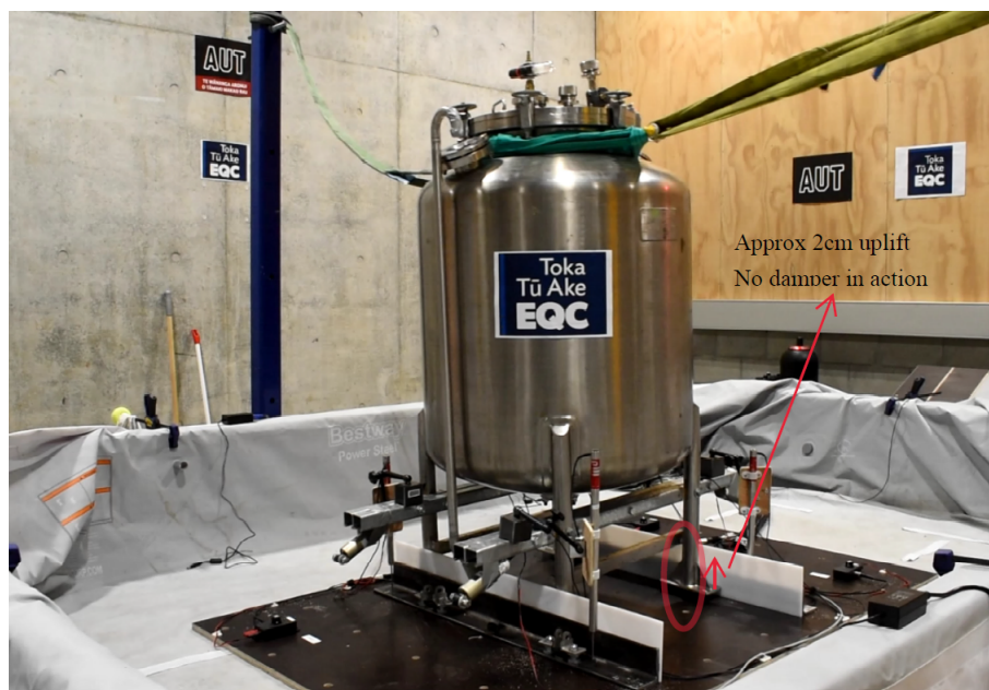
Figure 4.44: Experimental tests of the tank without MR dampers under applied ground motions - Christchurch 2011
