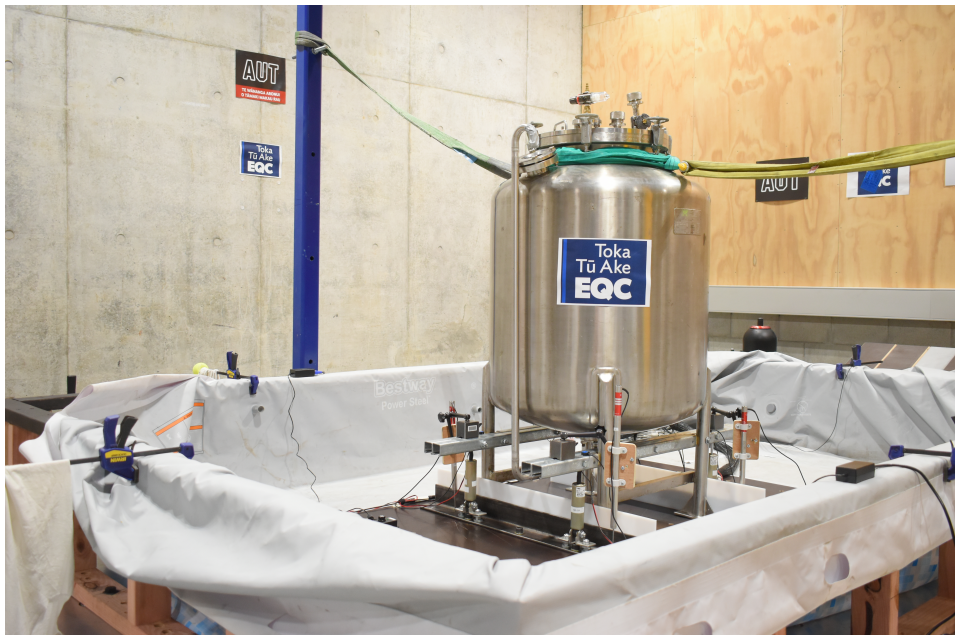
Figure 4.34: Experimental setup of the tank with MR dampers
