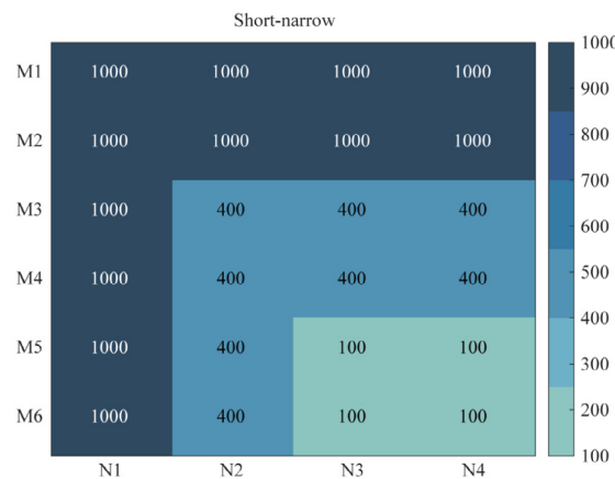
(e) Irradiance distribution of short-narrow shading for 6 \times 4 hybrid PV-TEG systems
