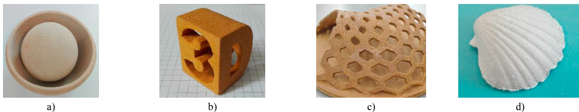
Fig. 8: test sample geometries a) (Miscanthus) ball/hollow hemisphere b) (Apricot stone) 3D symbol c) (Miscanthus) thin walled bridge structure d) (Sea shell) thin walled shell model
