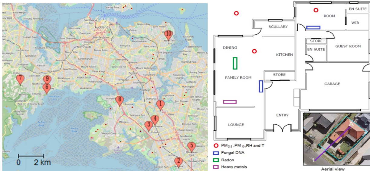
Fig. 1. Study house locations across Auckland / Typical floorplan and sensor layout.
