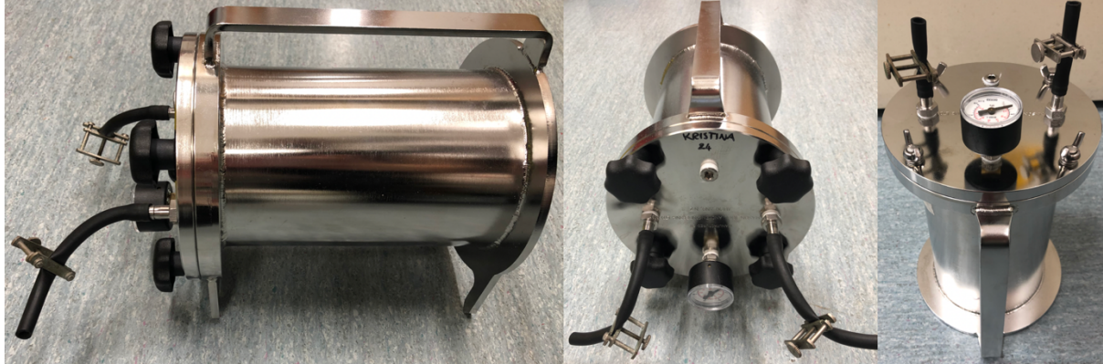
Figure 28: Anaerobic jars custom built by Mason Tool and Engineering Limited (Auckland, New Zealand). Has the option of agar plate vertical mode of operation as well as microwell plate horizontal mode of operation. Input and output valves allow gassing cylinder input through the Hungate gassing apparatus. Pressure gauge enables maintenance of a specific pressure during incubation.
