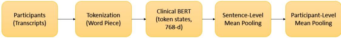
Figure 4.1: ClinicalBERT embedding pipeline. Each transcript segment was tokenized with WordPiece, encoded by ClinicalBERT, and the [CLS] state (768-d) was extracted. The segment vector is L2-normalised, regularised with Gaussian noise and modality dropout (training only), and projected into the 512-d latent space for graph fusion (Section 3.2). Author-created schematic
