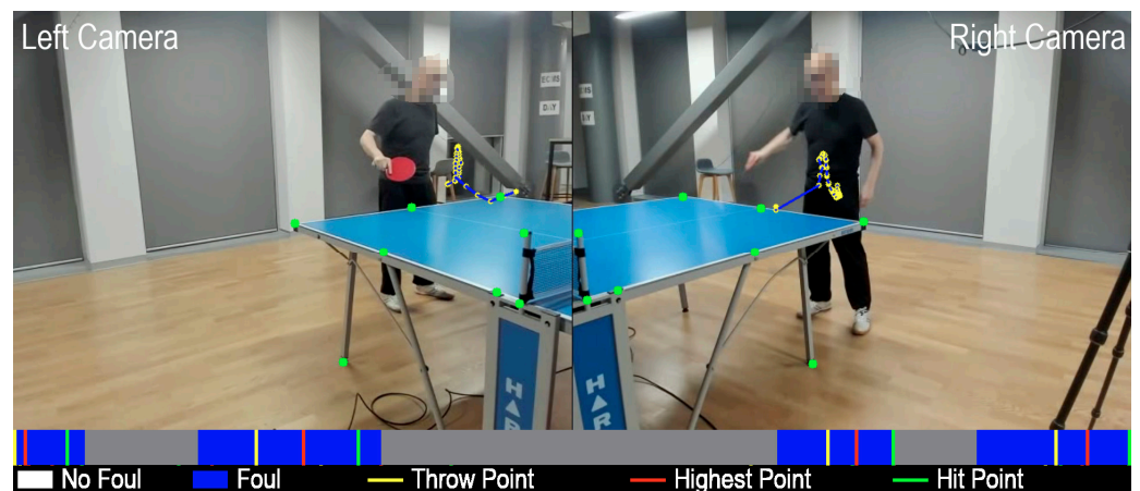
Figure 9. Video Segmentation Results: (Top) Synchronized left and right camera views showing key trajectory points during a table tennis serve. The throw point (yellow), highest point (red), and hit point (green) are marked to track the ball's trajectory. (Bottom) Segmented timeline showing frame classification as “No Foul” (gray) and “Foul” (blue), with transitions aligned to the serve events.
