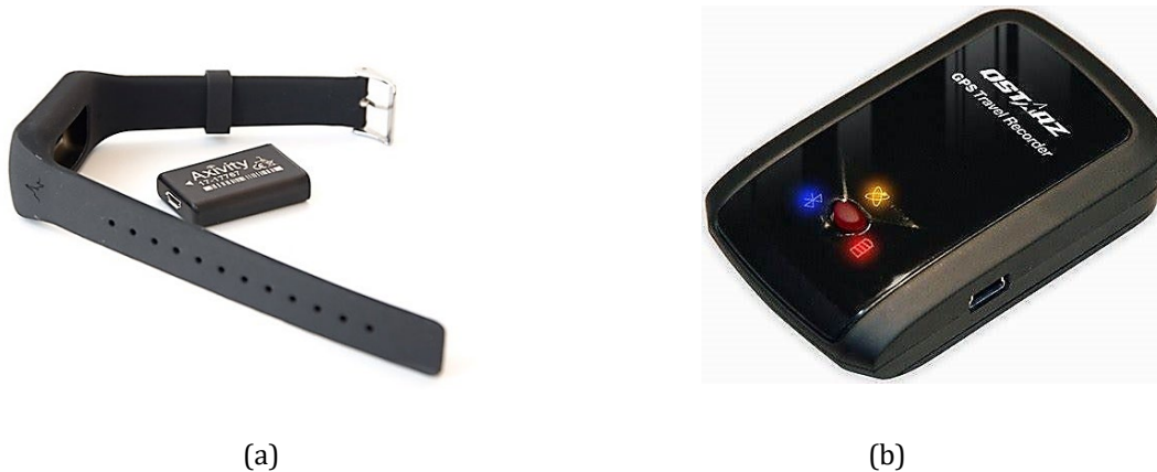
Figure 4-2. Equipment; (a): AX3 accelerometer, (b): QStarz BT-Q1000XT GPS
