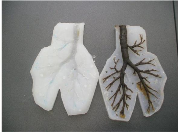
Figure 2.3 Second negative embedded into the mold
