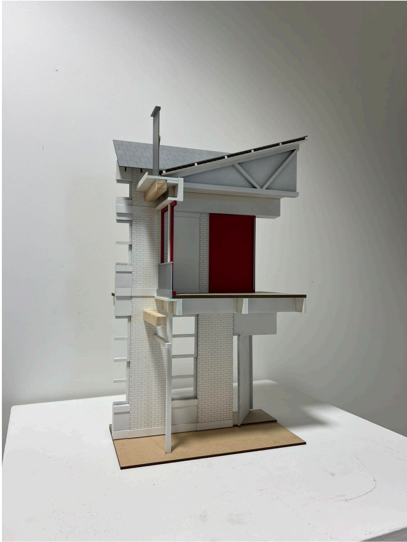
1:25 Sectional model of the opposing junction between the eastern addition and principal building
