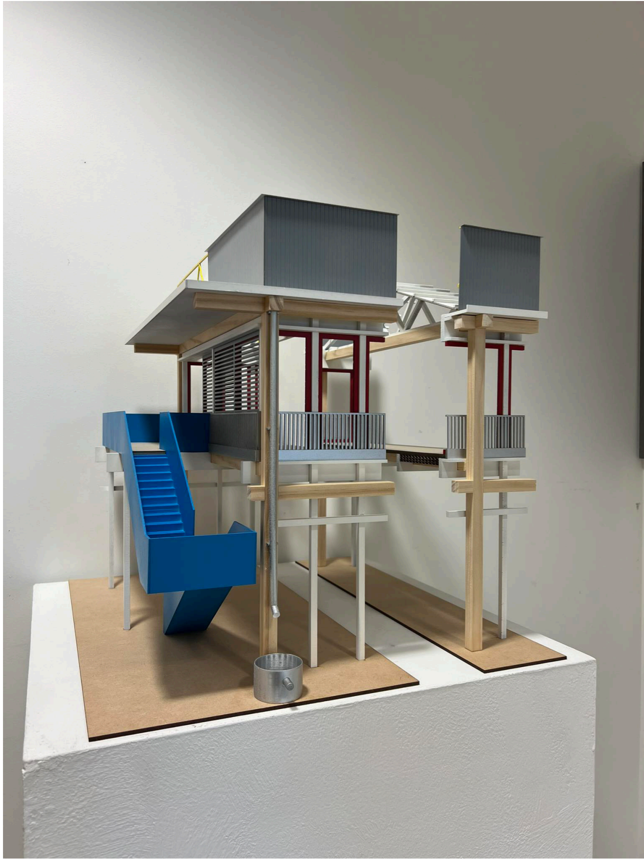
1:25 Sectional model of the eastern addition entry stair and typical 'core' short section
