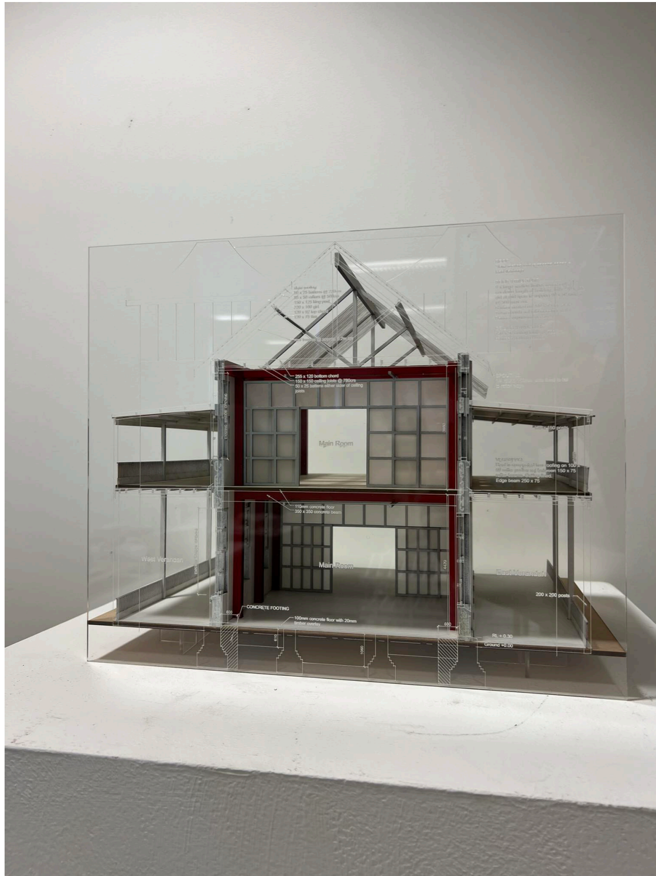
1:50 Sectional model of the principal building; section details, end 'towers', sub floor structure information and typical dimensions and materials etc engraved onto transparent material at point of section.
