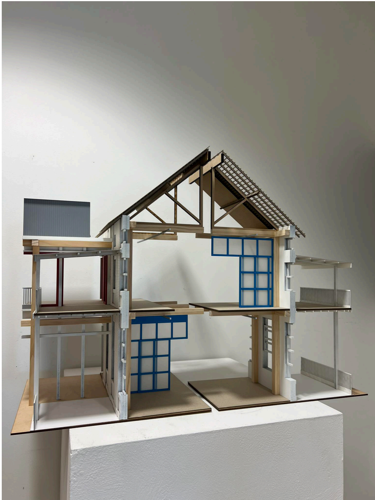
1:25 Sectional models of the critical junction 1 and principal building and verandah combined
