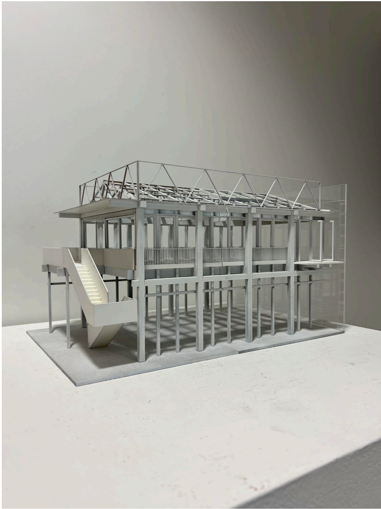
1:50 Study model 2 of the eastern addition construction split to show the short section
