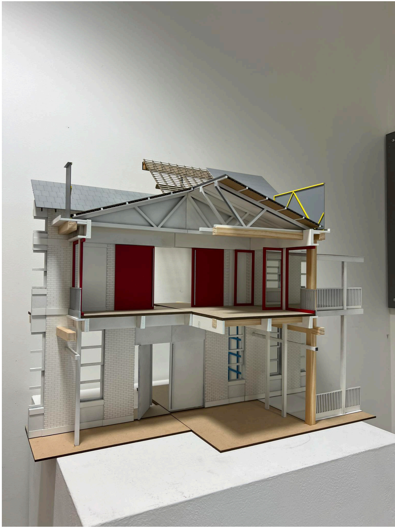
1:25 Sectional models of the critical junctions combined
