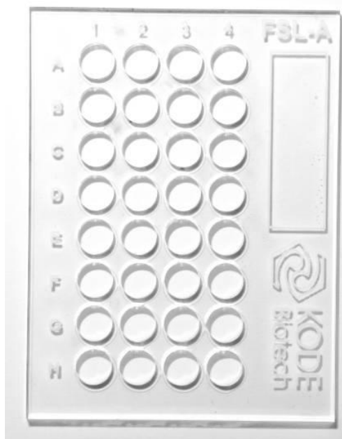
Fig. 2. Acrylic plate cut with 32 holes for reaction wells.
