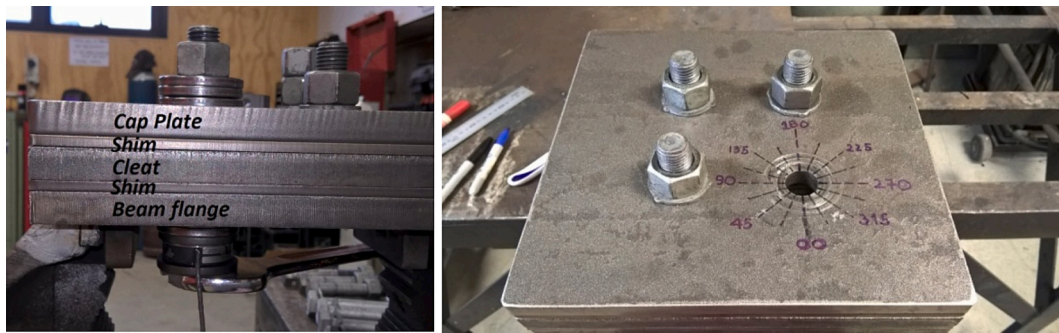
Fig. 9. Bolt tightening test setup (left) and measuring scale for the nut turn (right).
