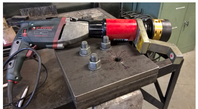
Fig. 1. Bolt tightening test setup.
