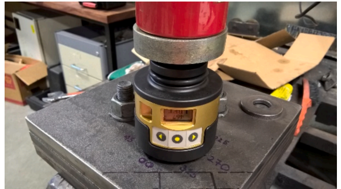
Fig. 7. The RAD smart socket.
