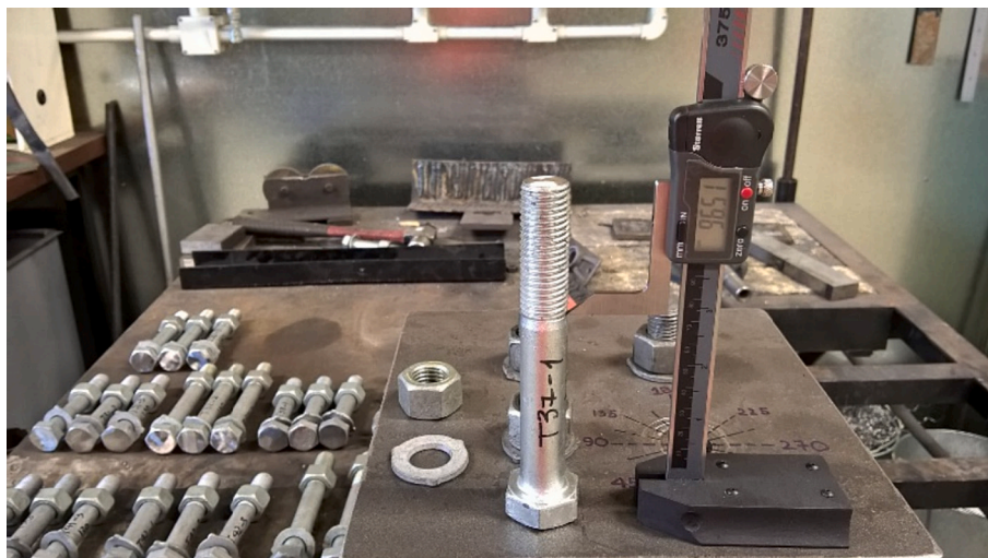
Fig. 6. The digital height gauge.
