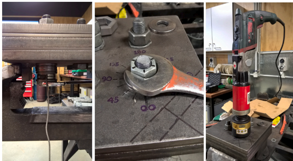
Fig. 10. The donut load cell (left), The standard spanner (middle), The electric torque multiplier with the smart socket (right).
