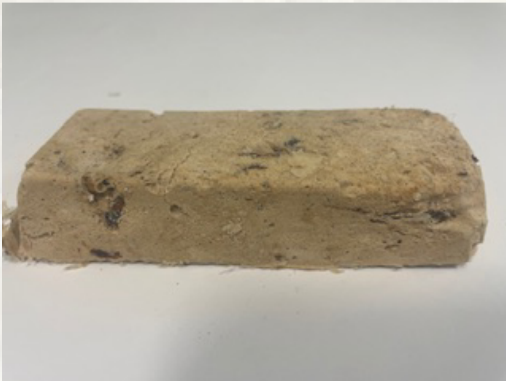
Figure 51: Bio-Resin encasing the sheep wool and seaweed
