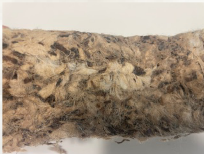
Figure 55: Visibly no crack in this bio brick
