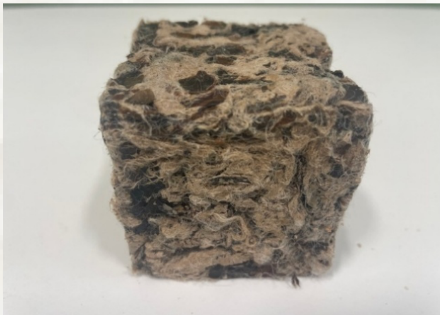
Figure 56: Final recipe of bio brick
