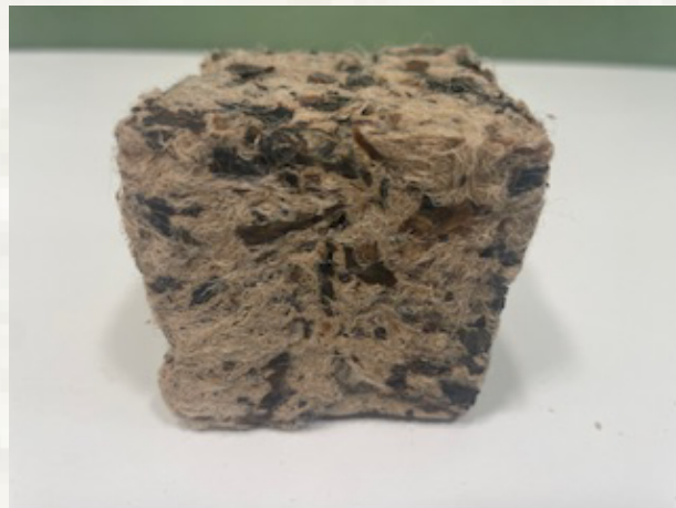
Figure 54: 20% Clay in this sample
