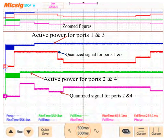
Fig. 16. Active power and quantified signals between ports.
