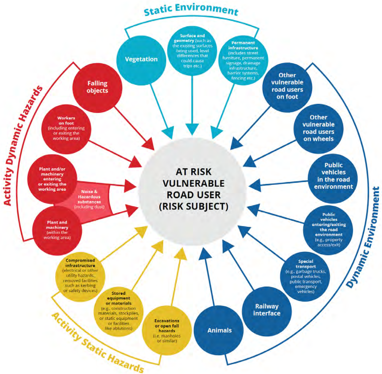
Figure 28 - Diagram of hazard sources for a VRU risk subject in a TTM setting 21
