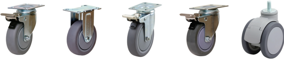
Figure 5. Casters used in the shake table tests. #1 to #5 from left to right.
