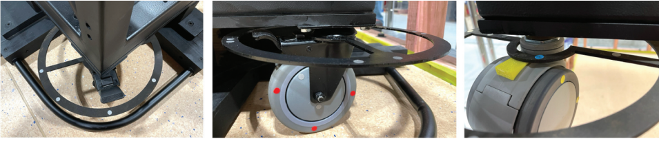
Figure 3. Reflective markers on a disk fixed to caster's fork (left), and disk mounted to the plate-type caster (middle) or stem-type caster (right).
