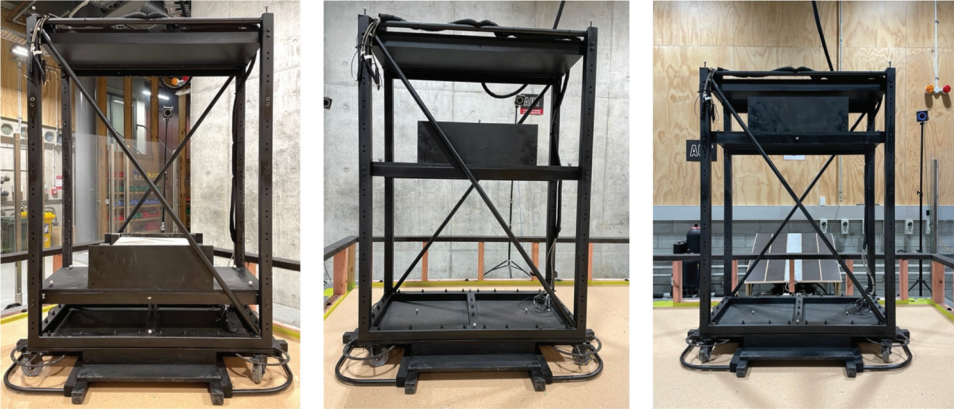
Figure 6. Adjustable center of mass by changing middle shelf position, “L,” “M,” and “H” from left to right.
